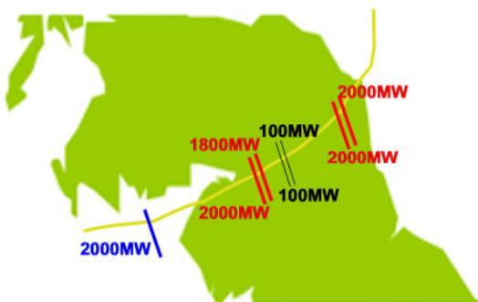
The adjacent diagram shows the circuits on the B6 constraint boundary and their capacities. The total capacity of the B6 is 10,000MW, 2,000MW of which relates to the HVDC link (shown in blue). As the HVDC link makes up 20% of the B6 boundary capacity, the desired B6 boundary flow on the HVDC link will be 1,200MW (20% of the B6 base boundary flow (6000MW)).
