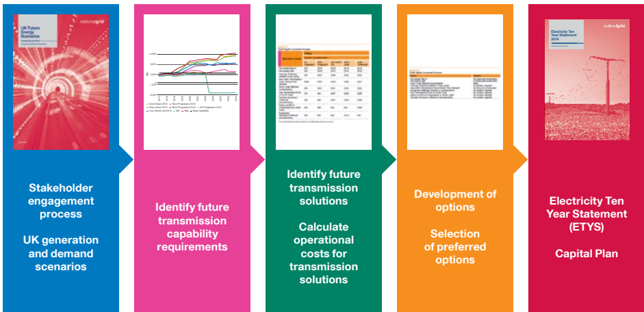
Figure 1.1 Network development process
