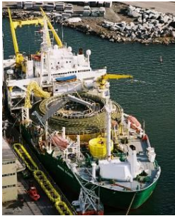
Figure E.9 Cable carousel on Nexans Skagerrak Image courtesy Nexans
