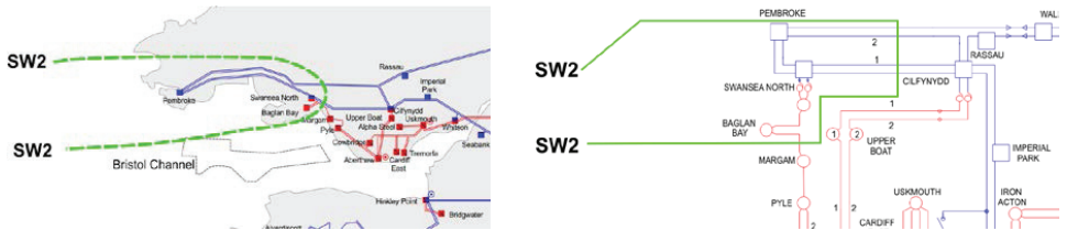
Figure SW2.1 Geographic and single line representation of boundary SW2
