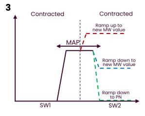
Unit must continue delivering until the end of the instruction, in line with the MAP, and must be ≥contracted MWs. Ramping starts in the second window
