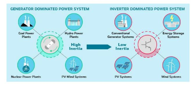
Wind turbine inertia - supporting the grid with active power (skeletontech.com)
