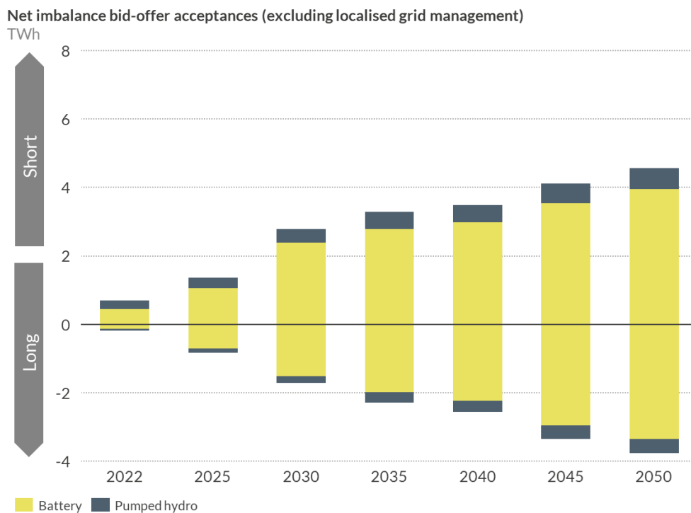
Figure 28: Forecast imbalance bid-offer acceptances of storage assets in the balancing mechanism
