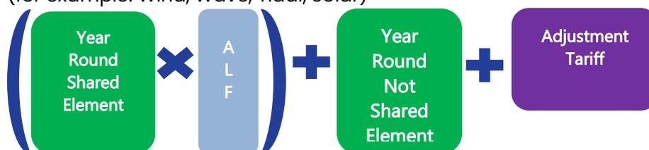
The **Peak** element reflects the cost of using the system at peak times. This is only paid by conventional and peaking generators; intermittent generators do not pay this element. The **Year Round Shared** and **Year Round Not Shared** elements represent the proportion of transmission network costs shared with other zones, and those specific to each particular zone respectively.
