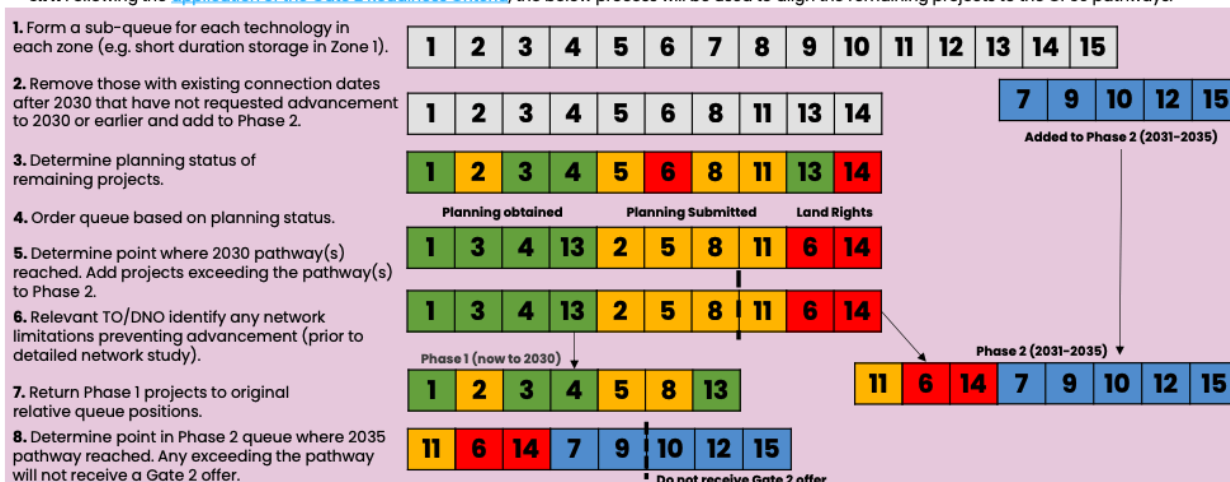
Figure 8: Aligning the queue to the CP30 pathways
