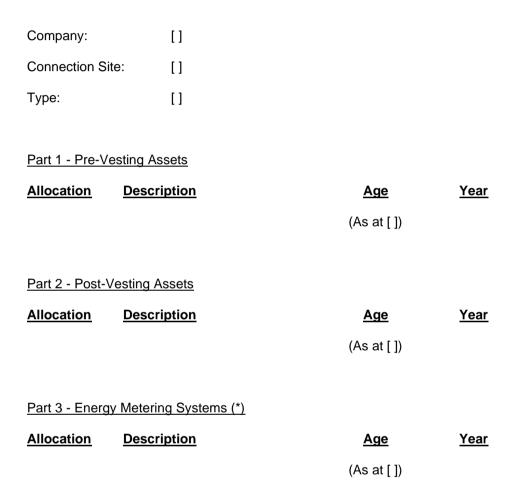
(\*) FMS, Energy Metering Systems - The Electronics components have a 15 year replacement period. The Non-Electronics components have a 40 year replacement period.
