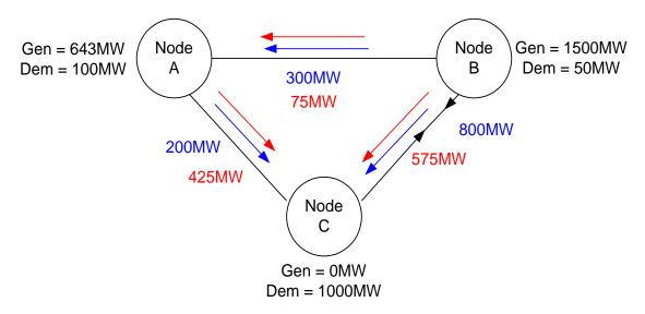
Therefore, circuits AB and BC are tagged as Peak Security and AC is tagged as Year Round.
