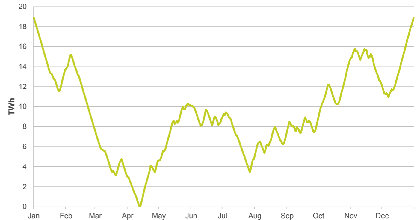
Figure ES.38: Hydrogen daily stock profile level in 2050 for Holistic Transition
