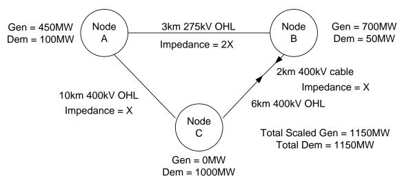
Assuming the same circuit impedances and expansion factors as used above in the Peak Security background, the DCLF transport algorithm calculates the base case power flows for Year Round background as follows:
