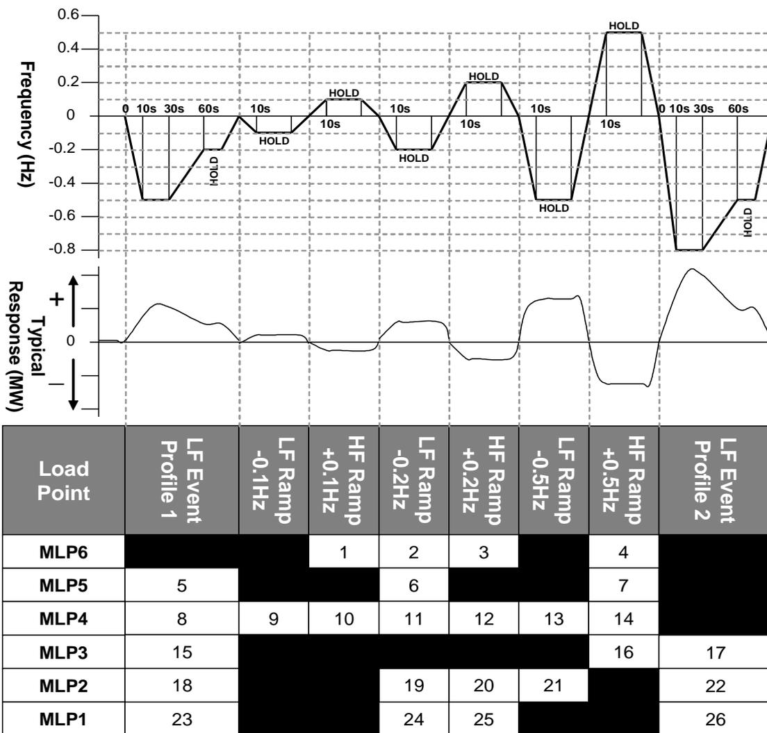
OC5.A.4.5. Figure 1 – Frequency response volume tests
