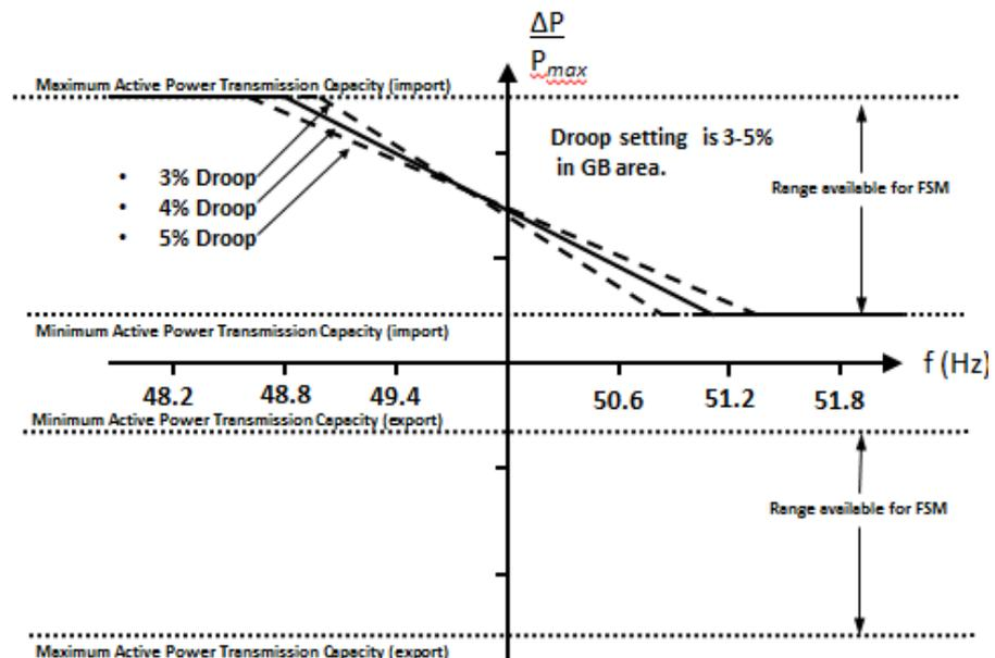
Figure 6.3.7.3.4(a) – **Active Power** frequency response capability of a **HVDC System** operating in **Frequency Sensitive Mode** (FSM).  $\Delta P$  is the change in active power output from the **HVDC System**.
