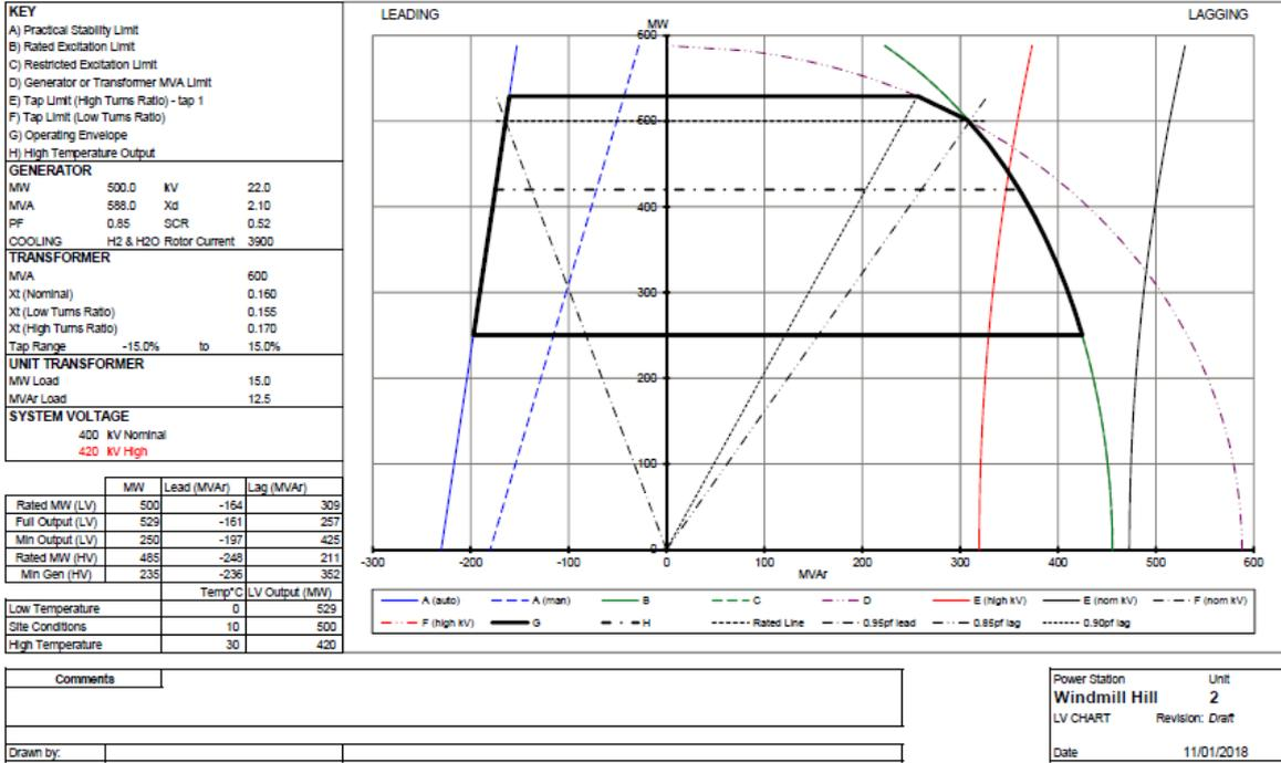
Synchronous Generating Unit Performance Chart within a Synchronous Power Generating Module
