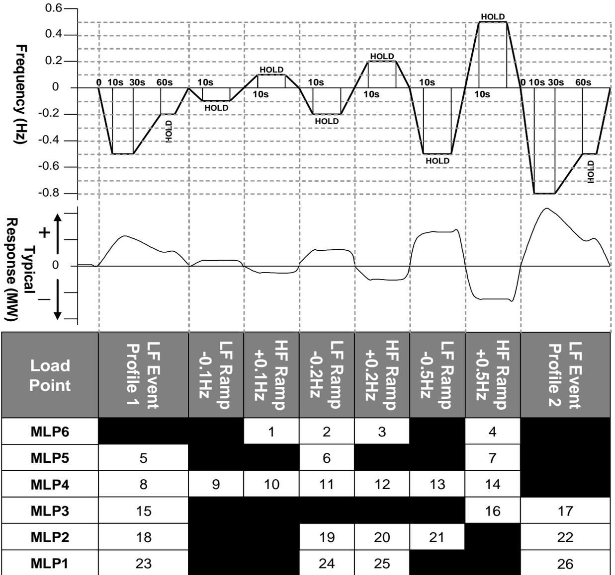
Figure 1: Frequency Response Capability FSM Ramp Response Tests
