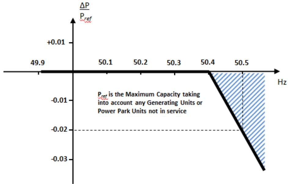
Figure ECC.6.3.7.1 –  $P_{ref}$  is the reference **Active Power** to which  $\Delta P$  is related and  $\Delta P$  is the change in **Active Power** output from the **Power Generating Module** (including **DC Connected Power Park Modules**) or **HVDC System**. The **Power Generating Module** (including **DC Connected Power Park Modules** or **HVDC Systems**) has to provide a negative **Active Power** output change with a droop of 10% or less based on  $P_{ref}$ .
