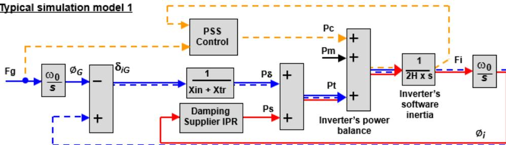
Figure PC.A.5.8.1 (a) Preferred simplified diagram of a **GBGF-I** with a **Power System Stabiliser “PSS”** that can add damping to the **GBGF-I’s** closed loop function shown by the solid red line and the dotted blue line.
