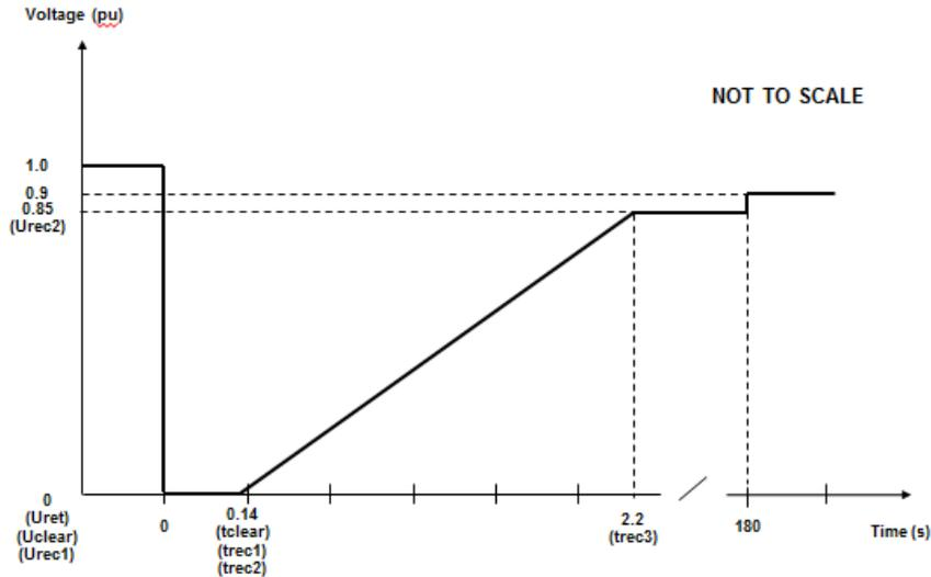
Figure ECC.6.3.15.6 - Voltage against time curve applicable to **Type D Power Park Modules** with a **Grid Entry Point** or **User System Entry Point** at or above 110kV, **DC Connected Power Park Modules** at the **HVDC Interface Point** or **OTSDUW Plant and Apparatus** at the **Interface Point**.
