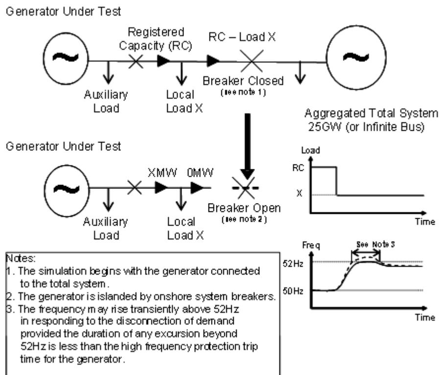
Figure CP.A.3.6.1 – Diagram of Load Rejection Study
