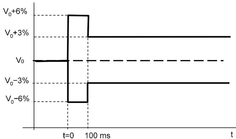
Figure ECC.6.1.7 (1) — Voltage characteristic for frequent events
