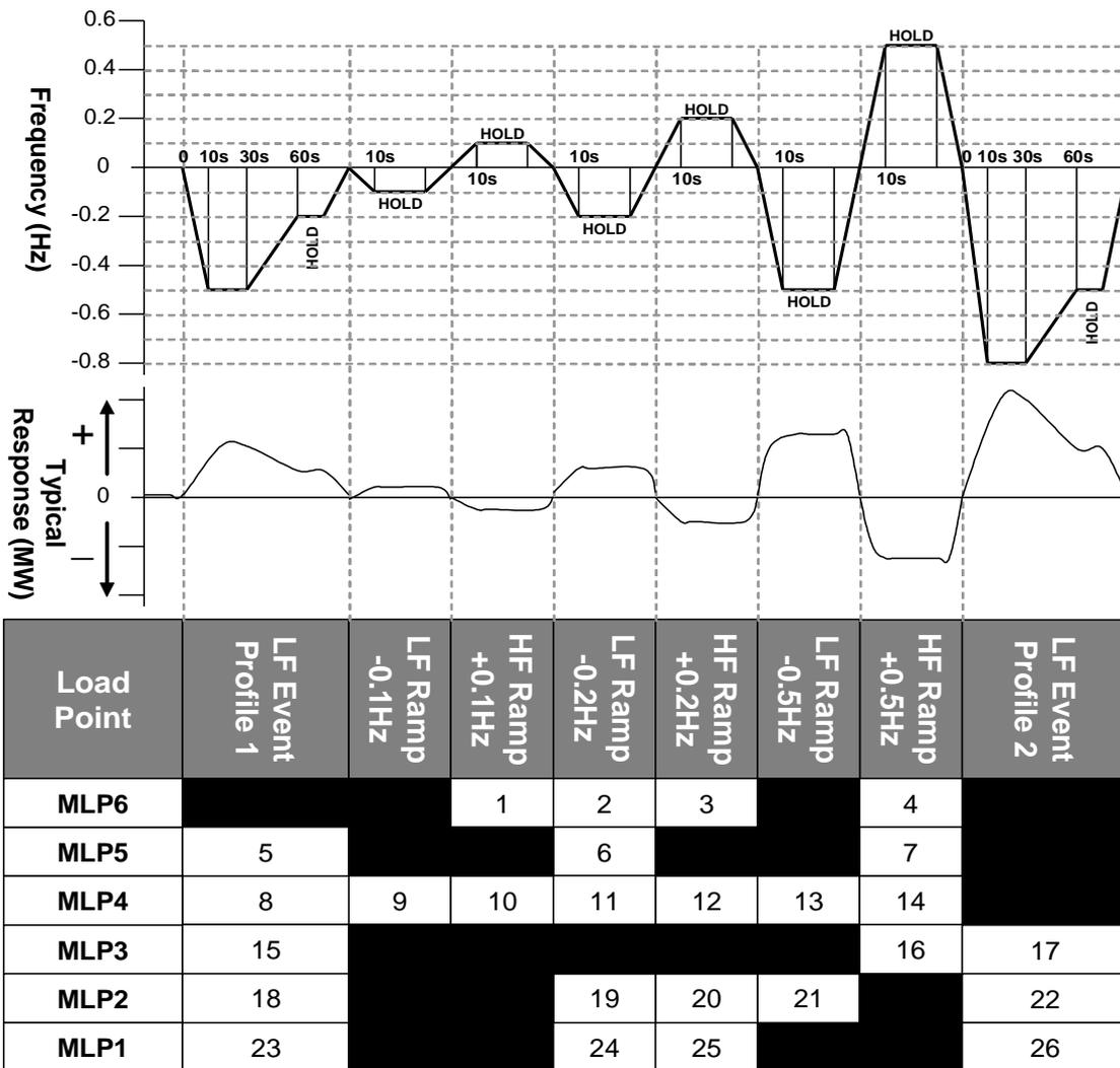
OC5.A.3.6. Figure 1 – Frequency response volume tests
