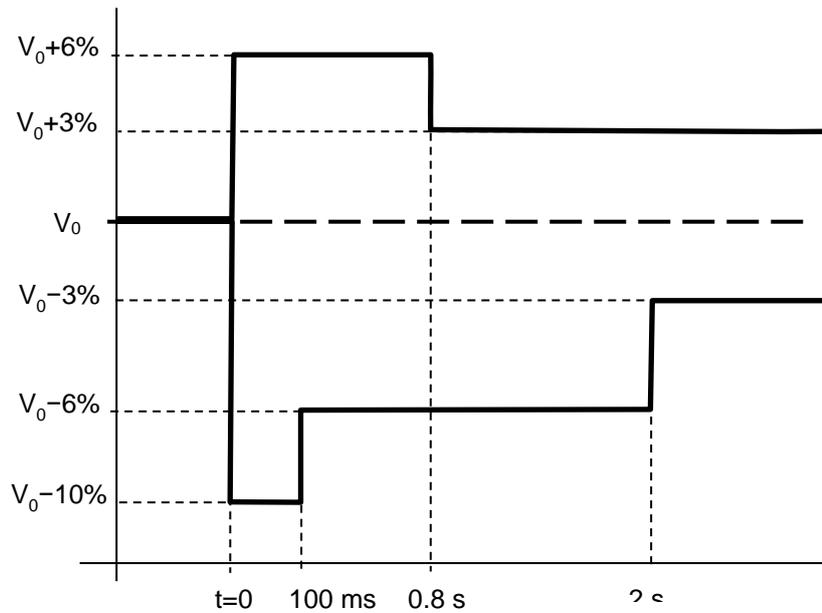
**Figure CC.6.1.7 (2) — Voltage characteristic for infrequent events**
