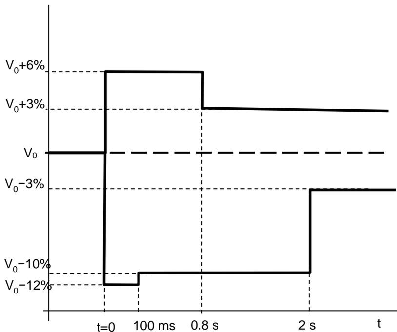
**Figure CC.6.1.7 (3) — Voltage characteristic for very infrequent events**
