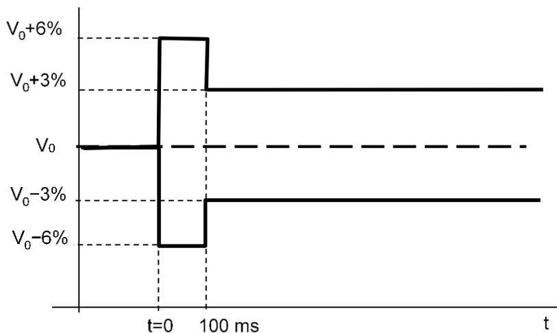
Figure CC.6.1.7 (1) — Voltage characteristic for frequent events
