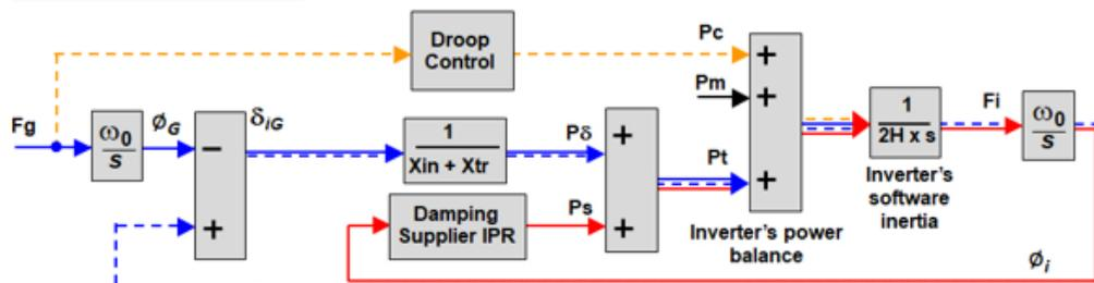
Figure PC.A.5.8.1 (b) – Preferred simplified diagram of a system with a droop control ability that can add **Control-Based Active Droop Power**. This diagram does not add extra closed loop damping to the **GBGF-I’s** closed loop function shown by the solid red line and the dotted blue line.
