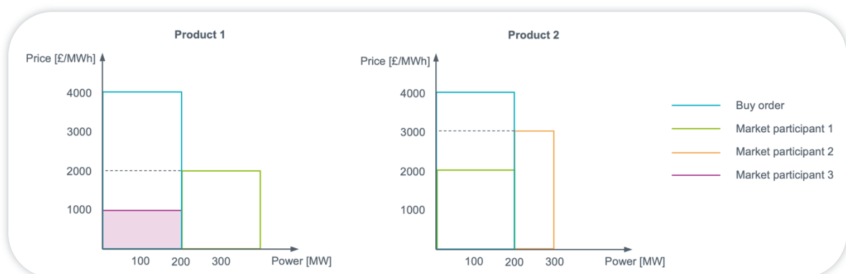
Figure 2 - Co-optimisation example: Market Participant 1 offers capacity for 2 products and the algorithm chooses for which product it is selected so that the welfare is maximised. The capacity offered by Market Participant 1 on Product 2 is selected by the algorithm as it produces a higher welfare.
