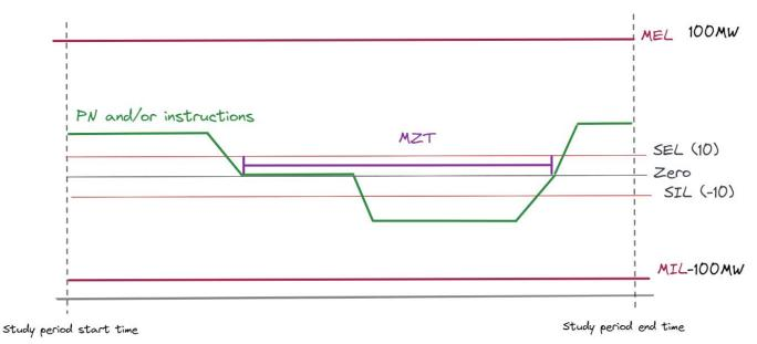
A bi-directional unit has moved to zero for MZT and then after the elapsed time move back in the same direction.
