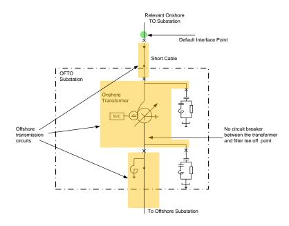
In comparison to Figure 1, with one less circuit breaker, the transformer circuit and the cable circuit connect directly to each other with no busbar in between.
