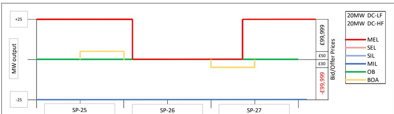
The MEL is redeclared to a positive value (+25MW in this example) when the unit is confident that the stored energy has returned to a level that would allow the unit to receive another offer acceptance of at least 15+2 minutes. In the example above, the issuing of a BM bid assists the unit in recovery of its stored energy.
