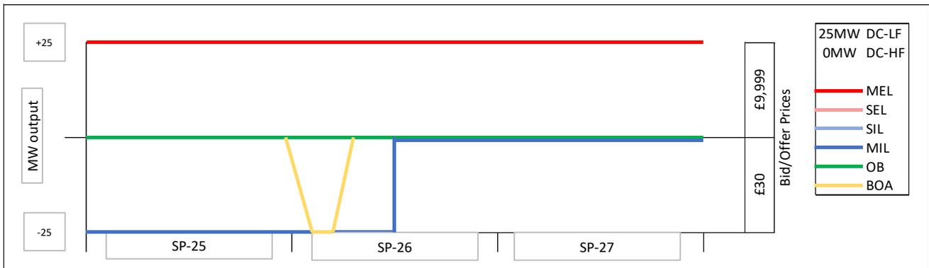
If the BOA was issued at maximum length for a battery BMU, the unit may re-declare its MIL at the point where the BOA ends as shown below for a 15+2min BOA.
