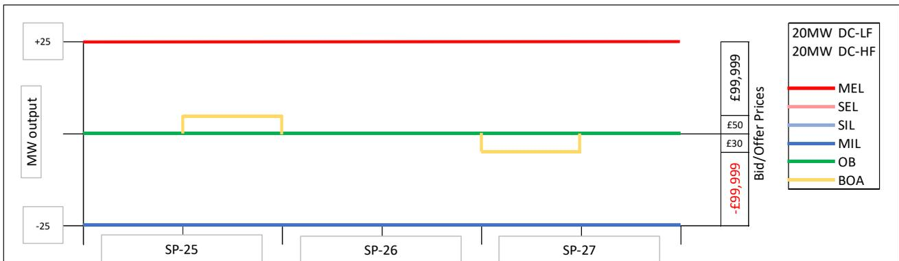
A simple case shown above where the issue of BOAs (one offer and one bid) does not require the unit to redeclare its MEL or MIL. The same BOA instructions are shown below but including a MEL to zero to reflect that the unit cannot accept any additional BOA offers.
