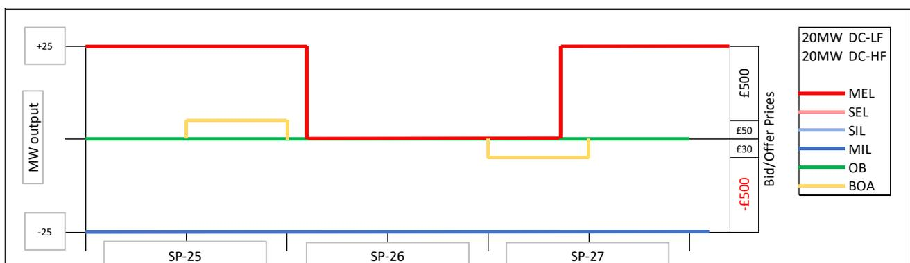
The MEL is redeclared to a positive value (+25MW in this example) when the unit is confident that the stored energy has returned to a level that would allow the unit to receive another offer
