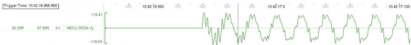
Figure 81: New Cumnock 132 kV voltage profile
