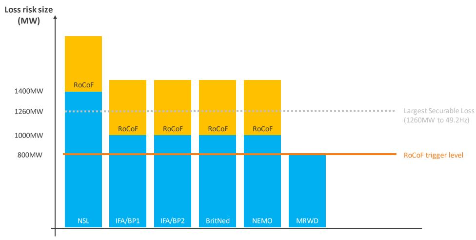
Dynamic Containment increases the size of the Largest Securable Loss
