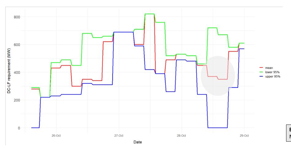
**EFA 4-5, 28**<sup>th</sup> **Oct 2021**Mean inertia = ~400MW DC-LF
