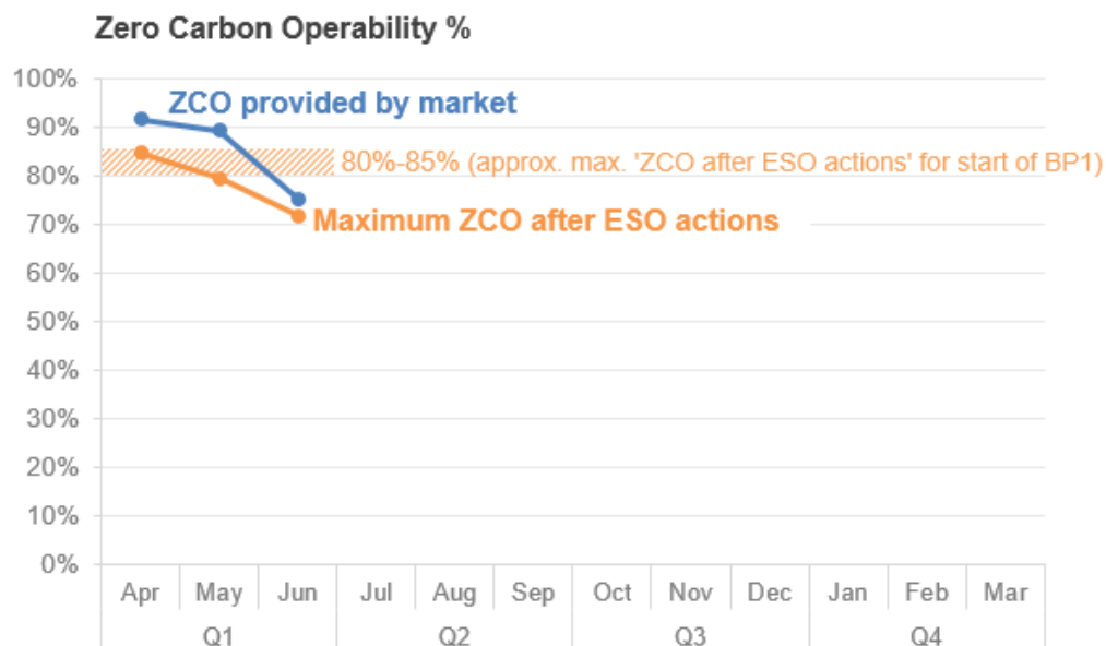
Figure 5: Maximum monthly ZCO% after ESO operational actions, versus ZCO provided by the market (during the settlement period when the maximum occurred)
