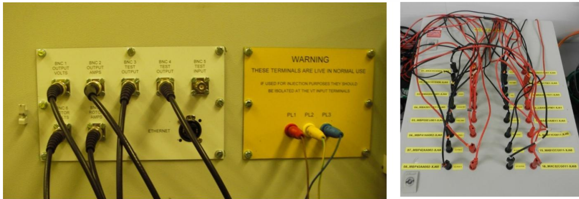
Figure 1 – Example of Compliance Test Signal Connections
