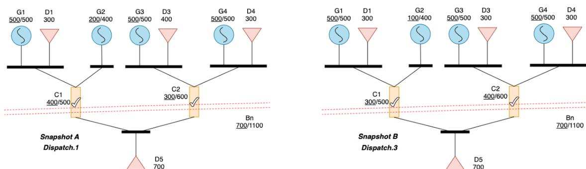
Figure 3.4. Comparison of dispatch results between two snapshots: Dispatch.1 for Snapshot A(left) and Dispatch.3 for Snapshot B (right)
