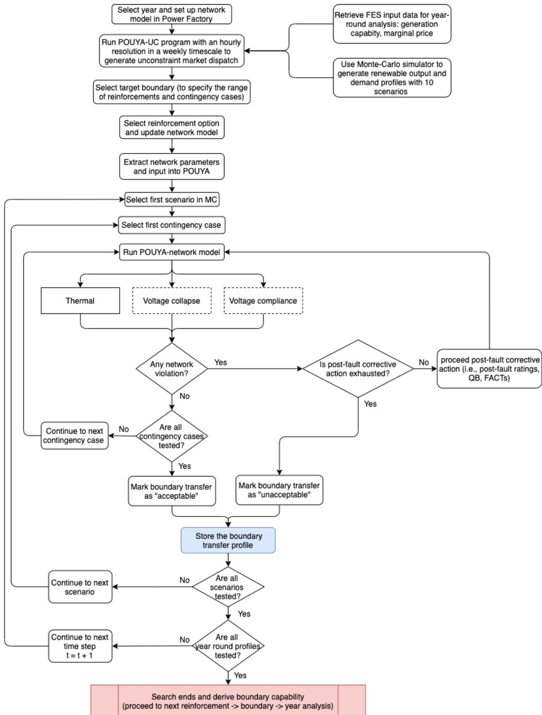
Figure 2.4. Workflow of evaluating boundary transfer profiles with a probabilistic method
