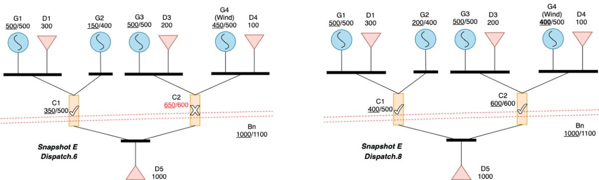
Figure 3.11. Comparison of dispatch results of Snapshot E: Dispatch.6 (original) and Dispatch.8 (renewable output curtailed).
