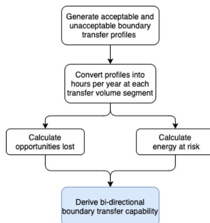
Figure 2.3. Probabilistic methodology in determining boundary transfer capability
