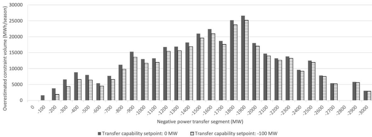
Figure 2.7. Overestimated volumes with 0 MW and -100 MW boundary transfer capability setpoints respectively
