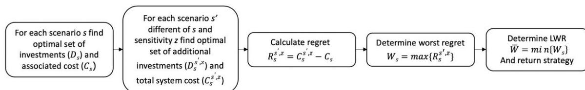
Figure 8.2. Steps for determination of LWR strategy in the transmission expansion stage of the ISP
