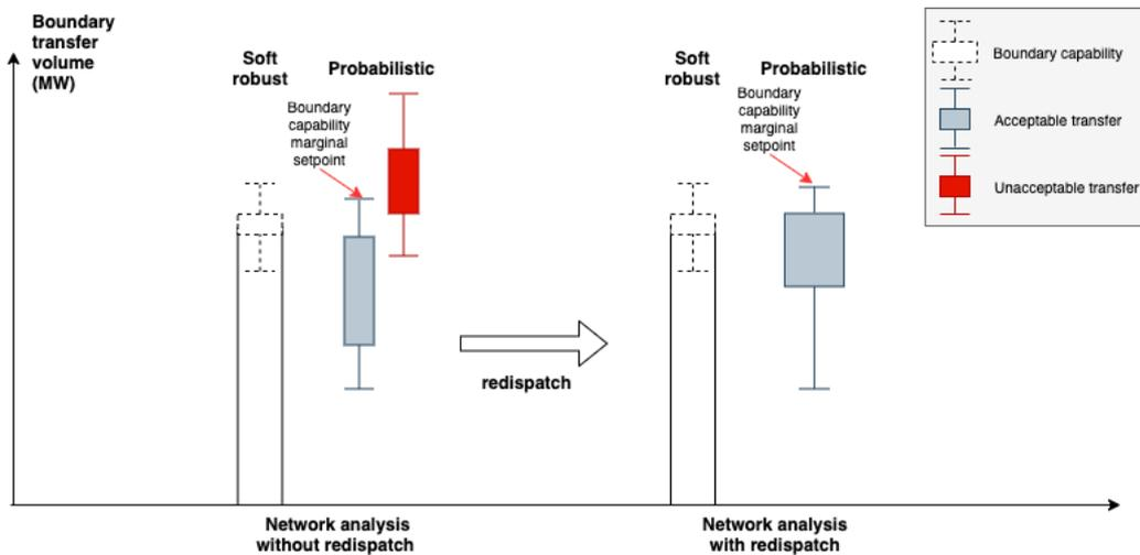
Figure 3.12. The distribution of acceptable and unacceptable transfer profiles before and after applying redispatch
