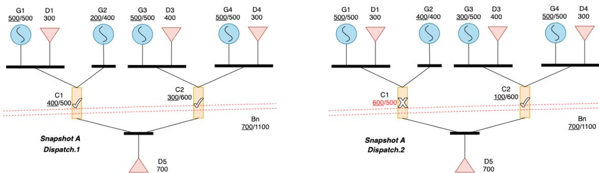
Figure 3.3. Two potential dispatch profiles of five bus system in Snapshot A: Dispatch.1(left) and Dispatch.2 (right)
