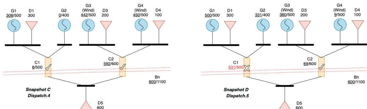
Figure 3.5. Five bus system configuration and two potential dispatch profiles (dynamic boundary capability with renewable generation)
