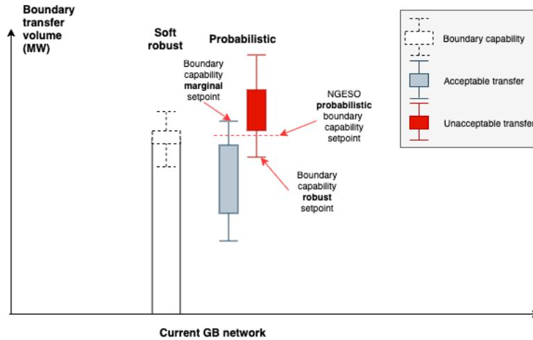
Figure 3.8. Illustration of boundary capability potential setpoints
