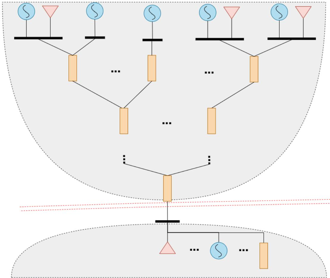
Figure 3.6. Illustration of boundary composition in a real power system
