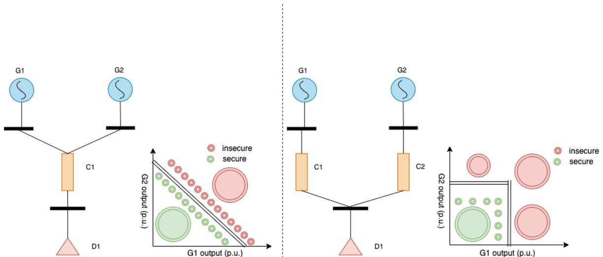
Figure 3.14. secure and insecure operating regions under different network topologies
