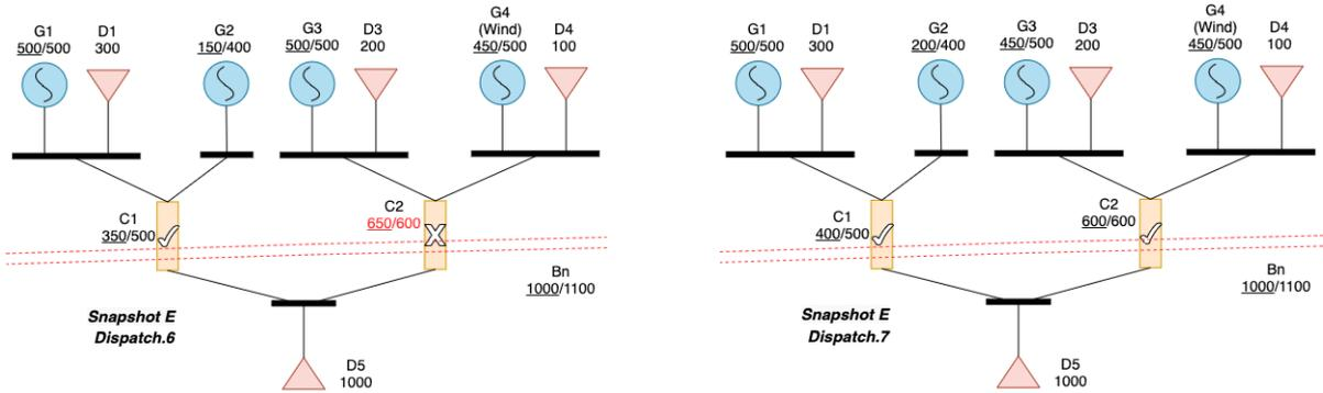
Figure 3.10. Comparison of dispatch results of Snapshot E: Dispatch.6 (original) and Dispatch.7 (conventional generator redispatched).
