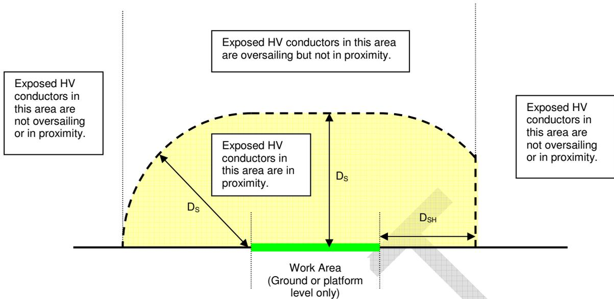
$D_s$  is the design clearance for safety (section clearance) specified in TS2.1 (RES).
