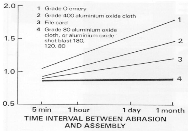
**Figure 5 - Initial Resistance of Bolted Aluminium Joints**
