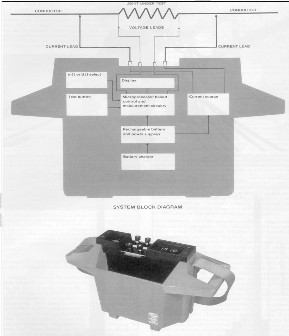
**Figure 4 - A typical Digital Micro Ohmmeter (DMO)**
