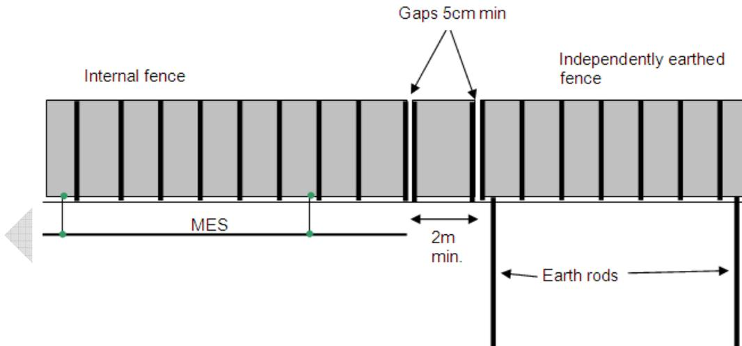
Figure 6 An example arrangement of separately earthed fences
