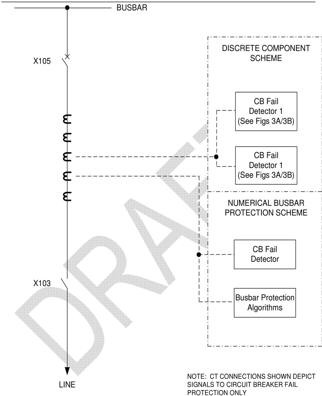
Figure 1: Typical CT Arrangement for Circuit Breaker Fail Protection for Busbar Stations - Feeder Circuit
