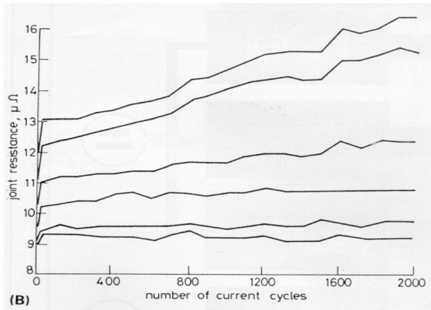
**Figure 6 - Load Cycle Performance measurements of Bolted Aluminium Joints with differing initial contact resistances**
