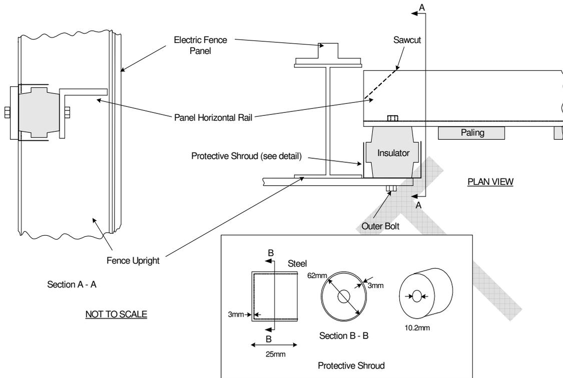
Figure 5 An example installation of insulating bushes on palisade fence
