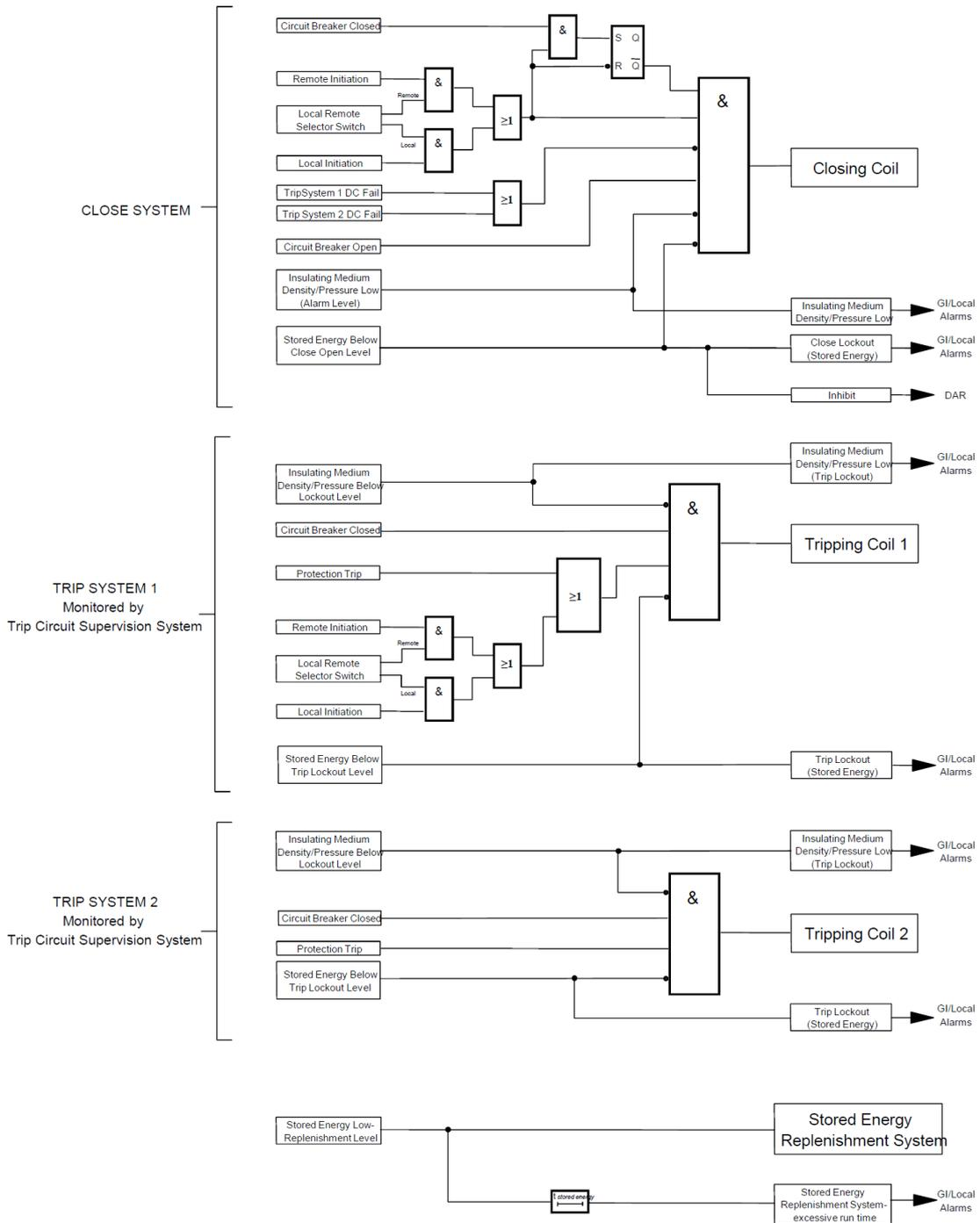
Attachment 4 - Three Phase Mechanism with Trip Lockout
