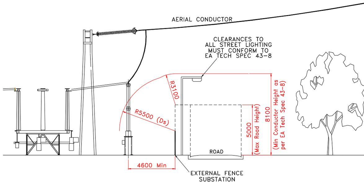
**Figure 1: Reduced Clearance to Substation Perimeter Fence (400kV Clearances Shown)**
