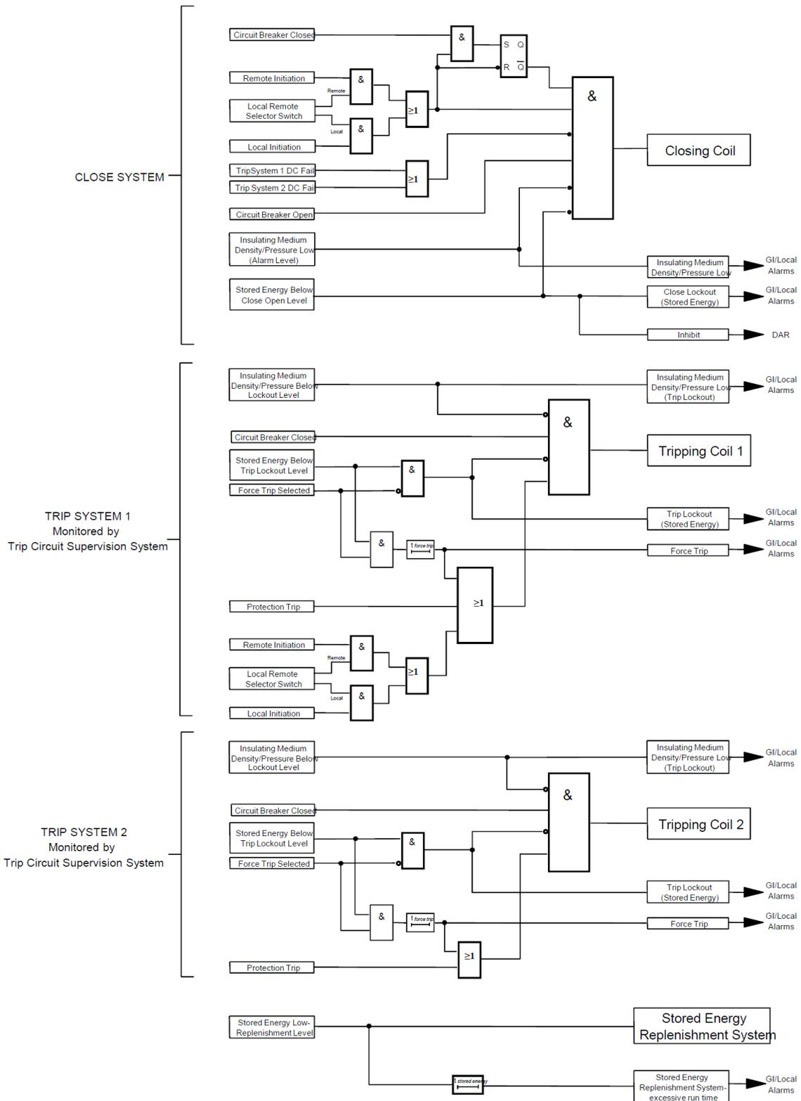
Attachment 3 - Three Phase Mechanism with Force Trip Facility
