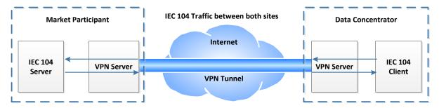
Once IEC 104 communication is established from NESO's IEC 104 client, the BM Participant will push the metering data to NESO.
