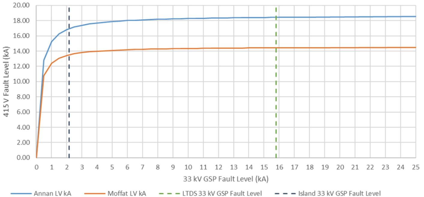
Figure 3.5 shows that for a 33kV fault level of ~2kA (provided by the anchor generator), the fault levels at 415V locations will be close to their normal values. Moreover, it can be seen that for 33kV fault levels greater than ~540A (30 MVA), the corresponding LV fault level will be ~65 per cent of its normal value or more. This means that a minimum fault level of ~30MVA (at a GSP 33kV busbar) is required to ensure correct downstream LV protection operation.
