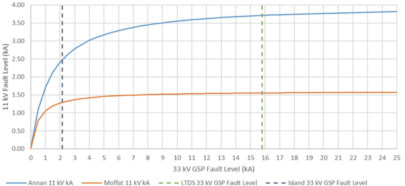
Figure 3.4 shows that for a 33kV fault level of ~2kA (provided by the anchor generator), the fault levels at 11kV locations will be around 60 per cent–85 per cent of the normal values.
