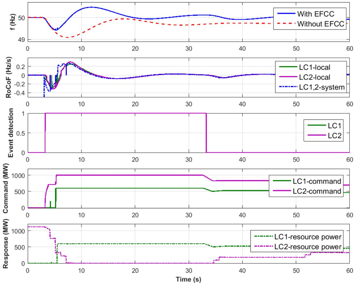
**Figure 37. Test 12: under-frequency event test results from LCs**
