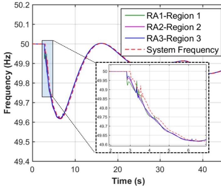
Figure 90. Data recorded in the RAs in the under-frequency test in Test 11
