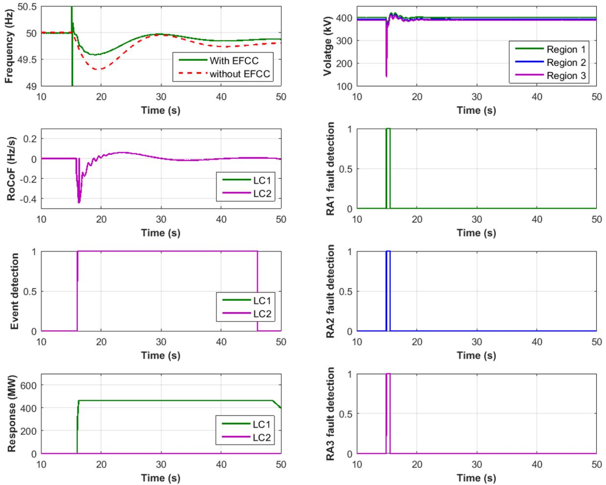
**Figure 73. Test results for a loss of generation event following Ph-Ph fault in Region 3**
