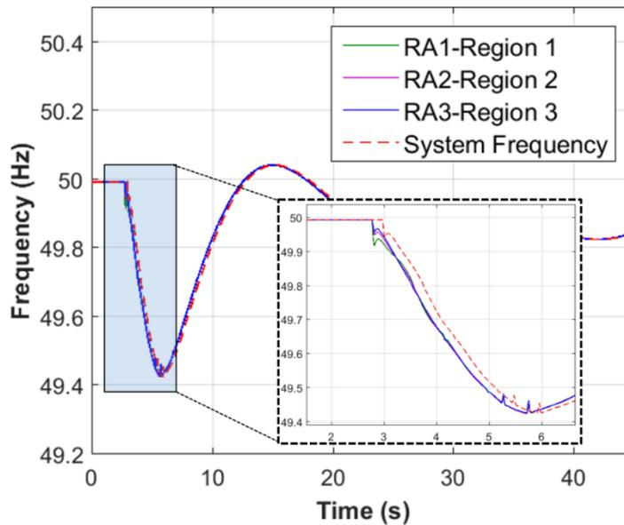
Figure 94. Data recorded in the RAs in the under-frequency test in Test 15
