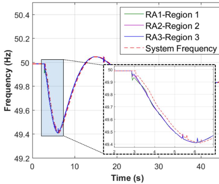
Figure 93. Data recorded in the RAs in the under-frequency test in Test 14
