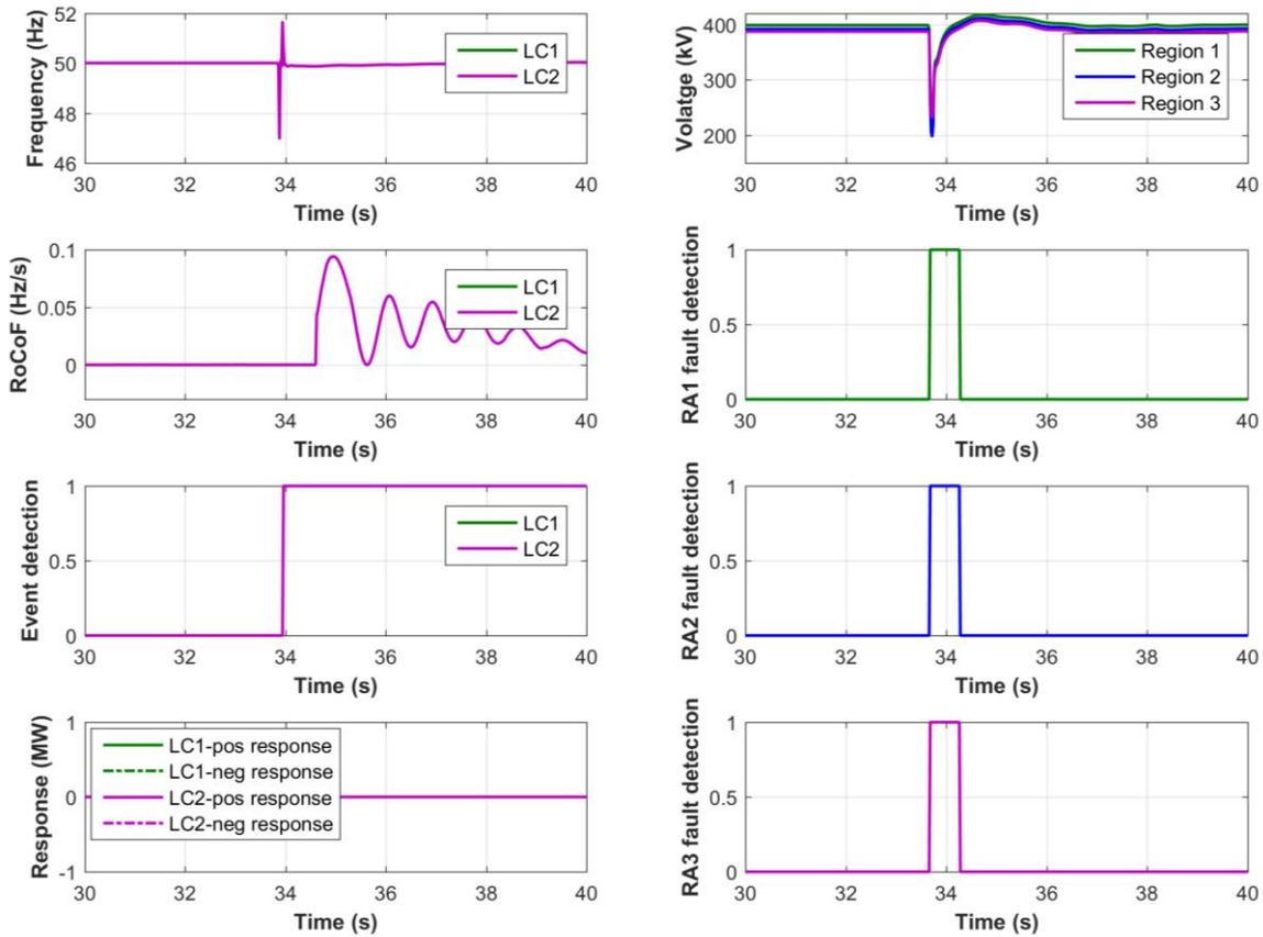
Figure 61. Test results for a 3Ph-E fault in Region 2
