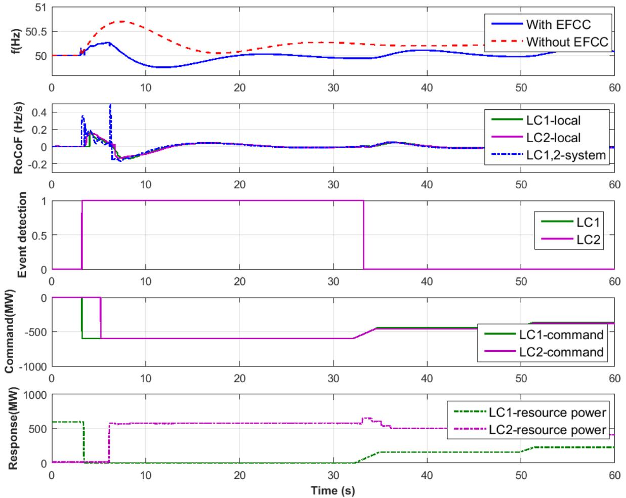
**Figure 17. Test 5: over-frequency event test results from LCs**
