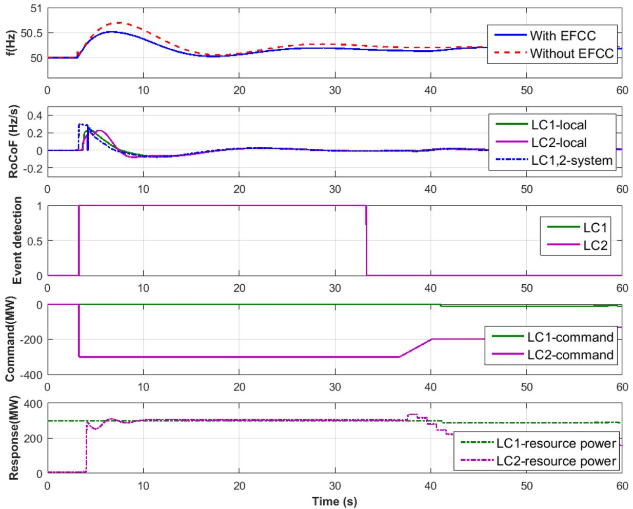
**Figure 5. Test 1: over-frequency event test results from LCs**
