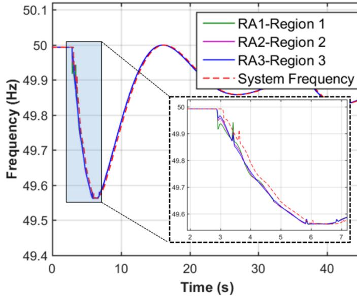
Figure 82. Data recorded in the RAs in the under-frequency test in Test 3
