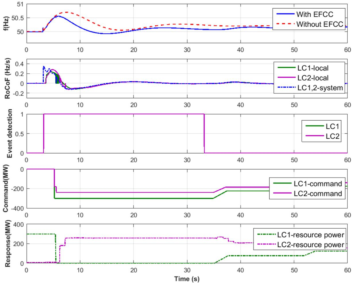
**Figure 44. Test 14: over-frequency event test results from LCs**
