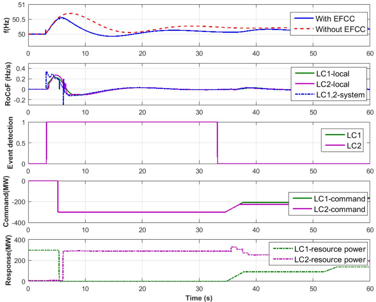
**Figure 47. Test 15: over-frequency event test results from LCs**
