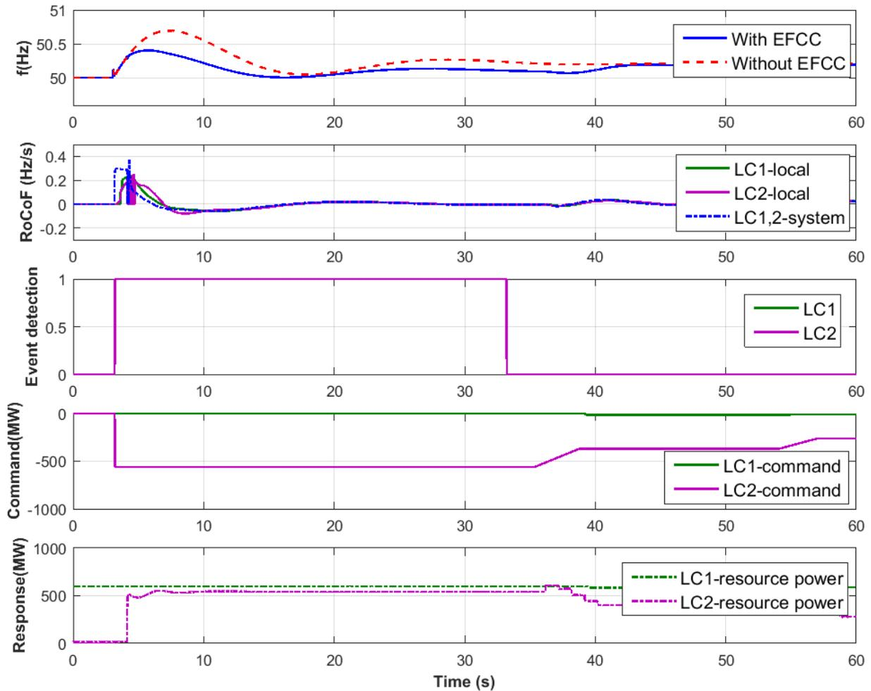
**Figure 14. Test 4: over-frequency event test results from LCs**
