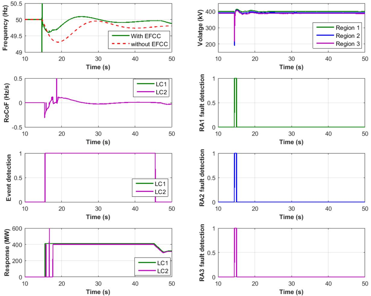
**Figure 71. Test results for a loss of generation event following 3Ph-E fault in Region 2**
