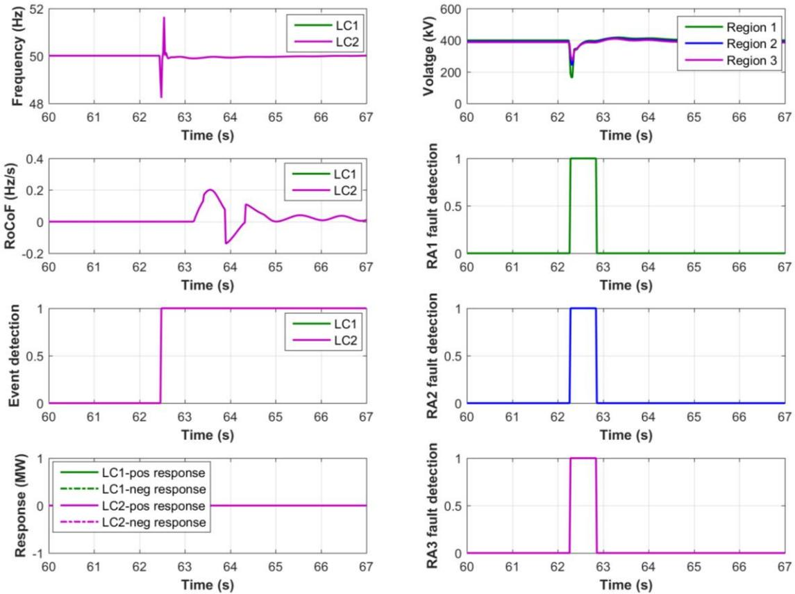
Figure 57. Test results for a 3Ph-E fault in Region 1
