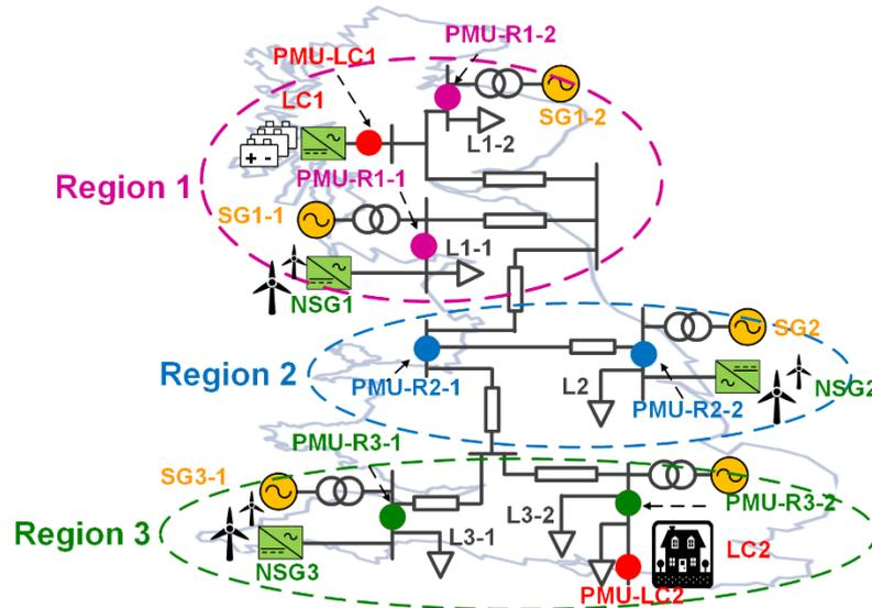
**Figure 2. Schematic of the reduced GB transmission network model in RTDS**
