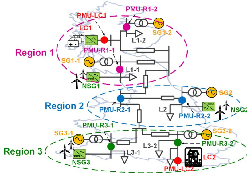
Figure 76. Schematic of the RTDS GB reduced transmission network model
