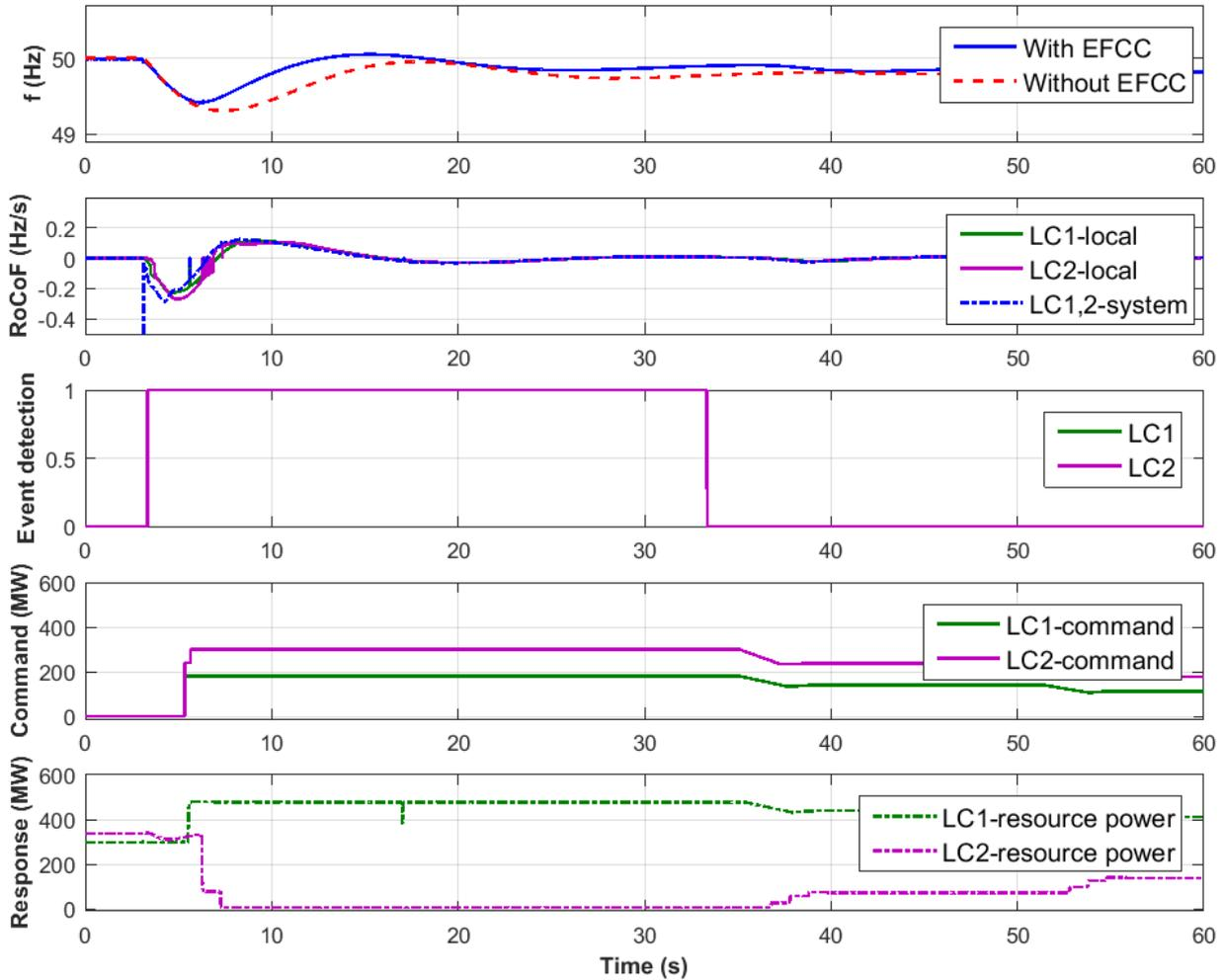
**Figure 43. Test 14: under-frequency event test results from LCs**
