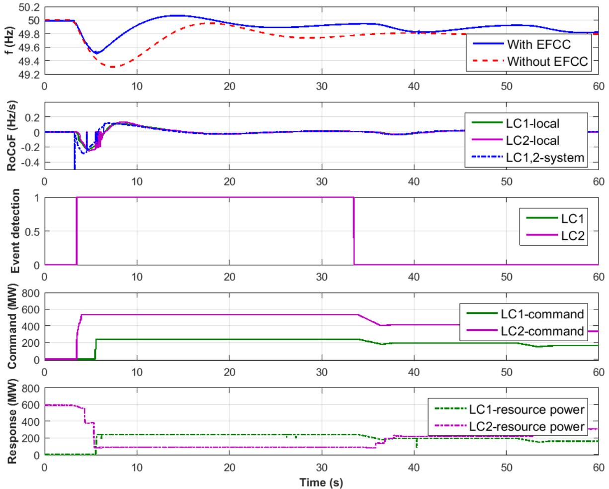
**Figure 13. Test 4: under-frequency event test results from LCs**
