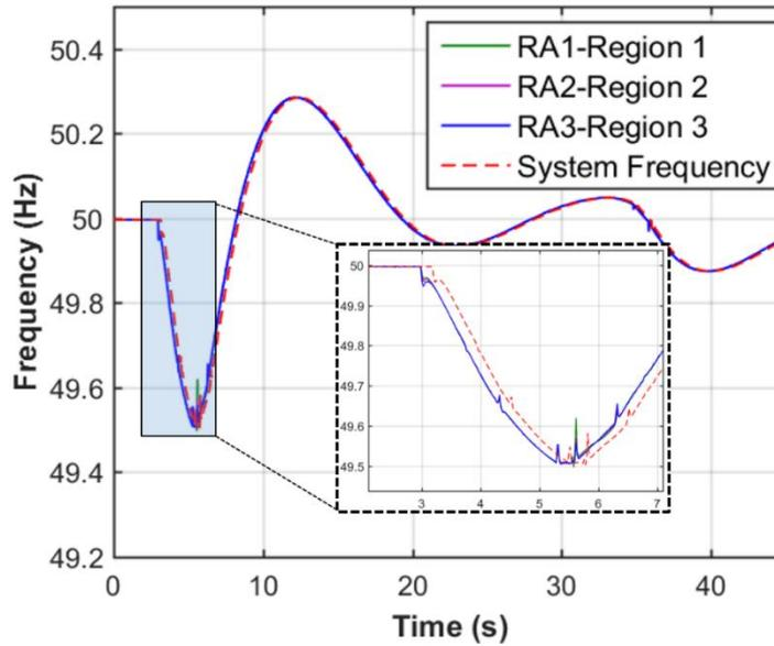
Figure 85. Data recorded in the RAs in the under-frequency test in Test 6
