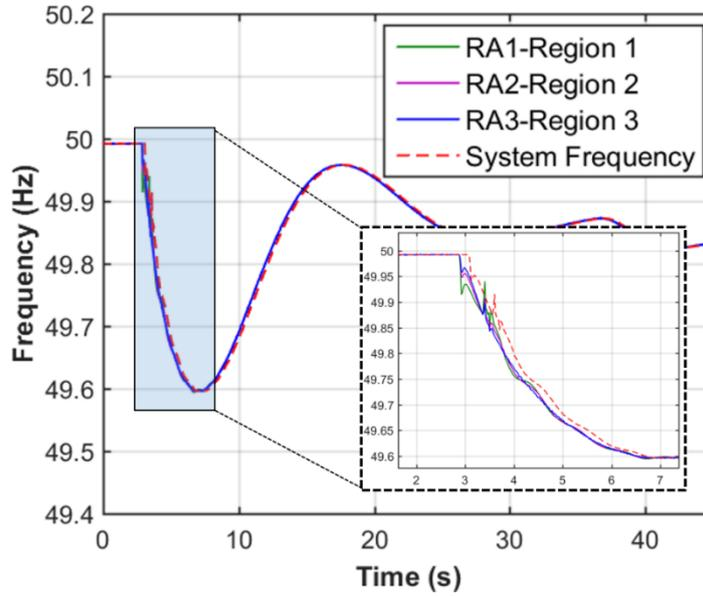
Figure 86. Data recorded in the RAs in the under-frequency test in Test 7
