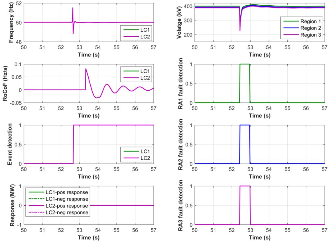
**Figure 64. Test results for a Ph-Ph fault in Region 3**
