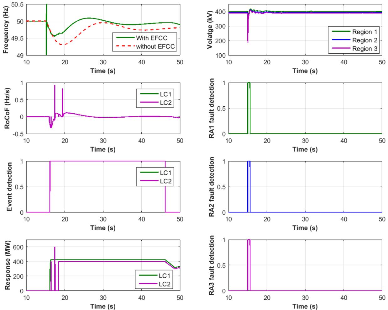
**Figure 74. Test results for a loss of generation event following 3Ph-E fault in Region 3**
