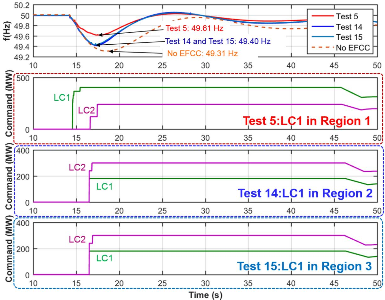
Figure 51. Comparison of under-frequency tests in Test 5, 14 and 15
