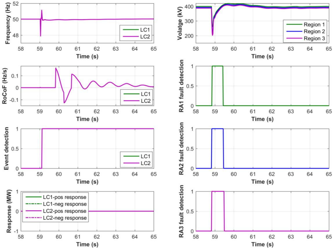
**Figure 65. Test results for a 3Ph-E fault in Region 3**
