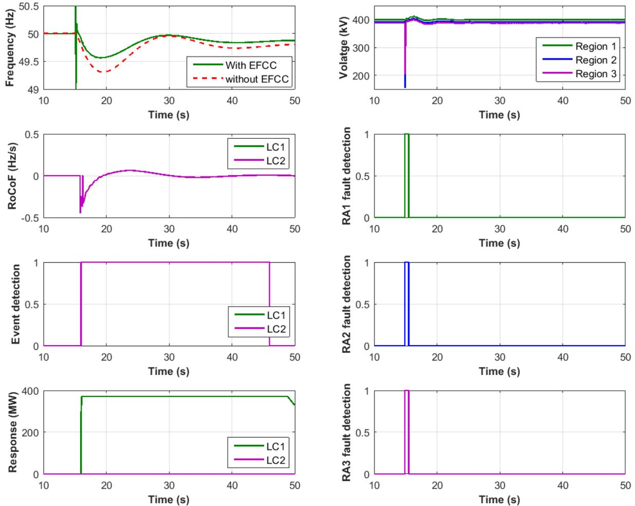
**Figure 70. Test results for a loss of generation event following Ph-Ph fault in Region 2**
