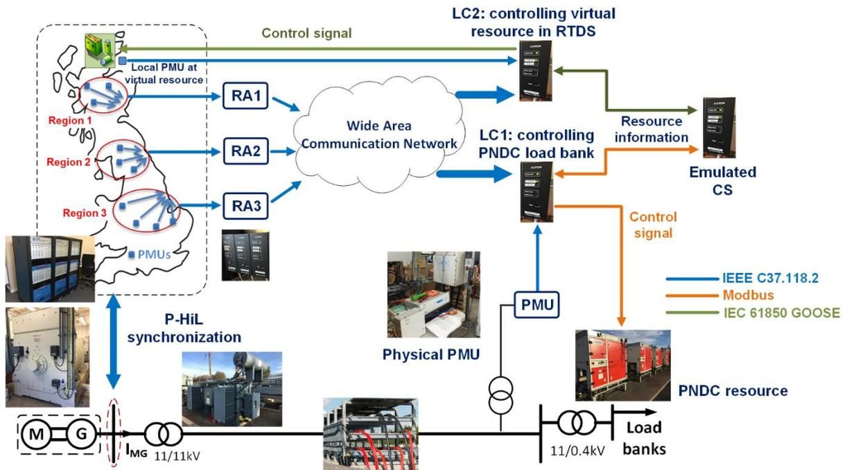
**Figure 1. P-HiL testbed for testing EFCC’s wide area operational mode**
