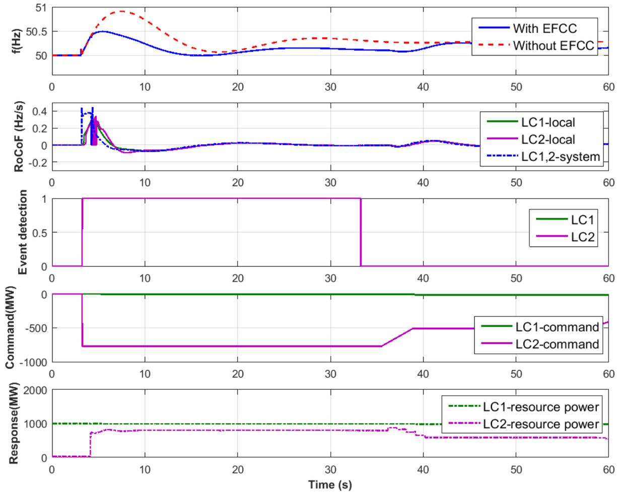
**Figure 38. Test 12: over-frequency event test results from LCs**
