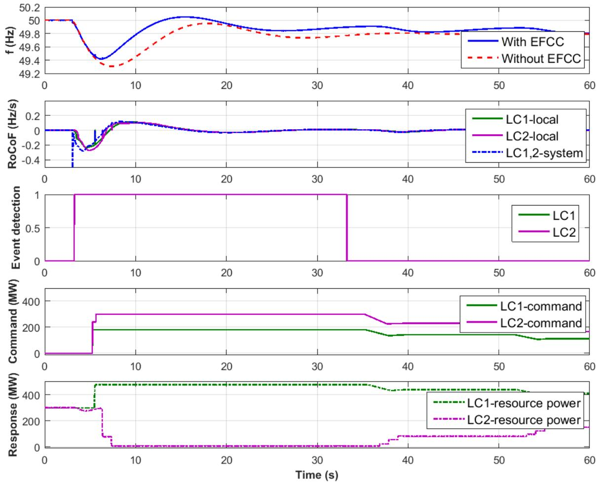
**Figure 7. Test 2: under-frequency event test results from LCs**
