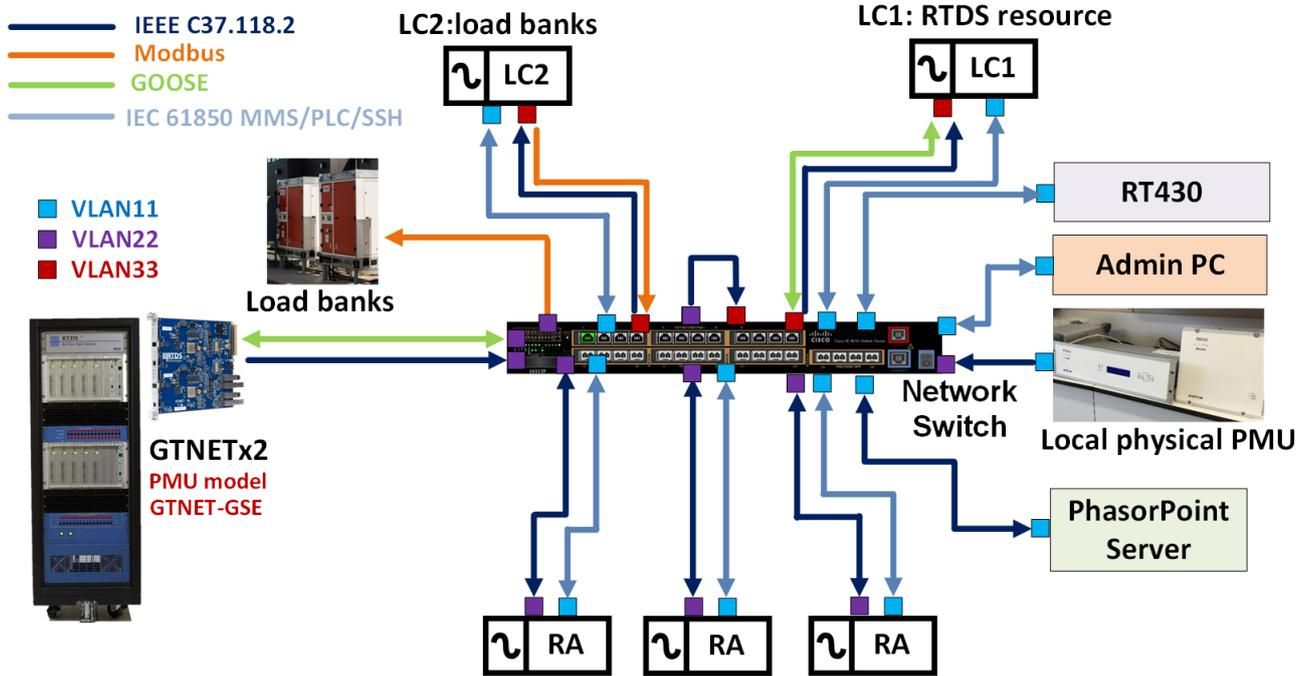
Figure 75. Setup of communication links
