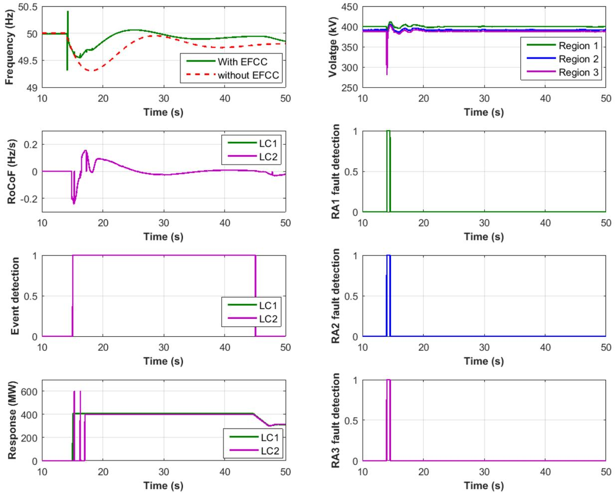
**Figure 72. Test results for a loss of generation event following Ph-E fault in Region 3**
