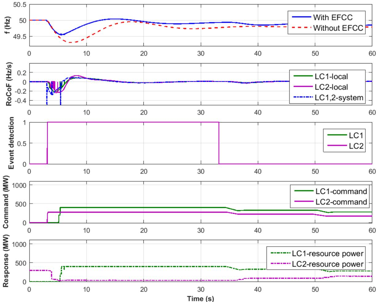
Figure 31. Test 10: under-frequency event test results from LCs
