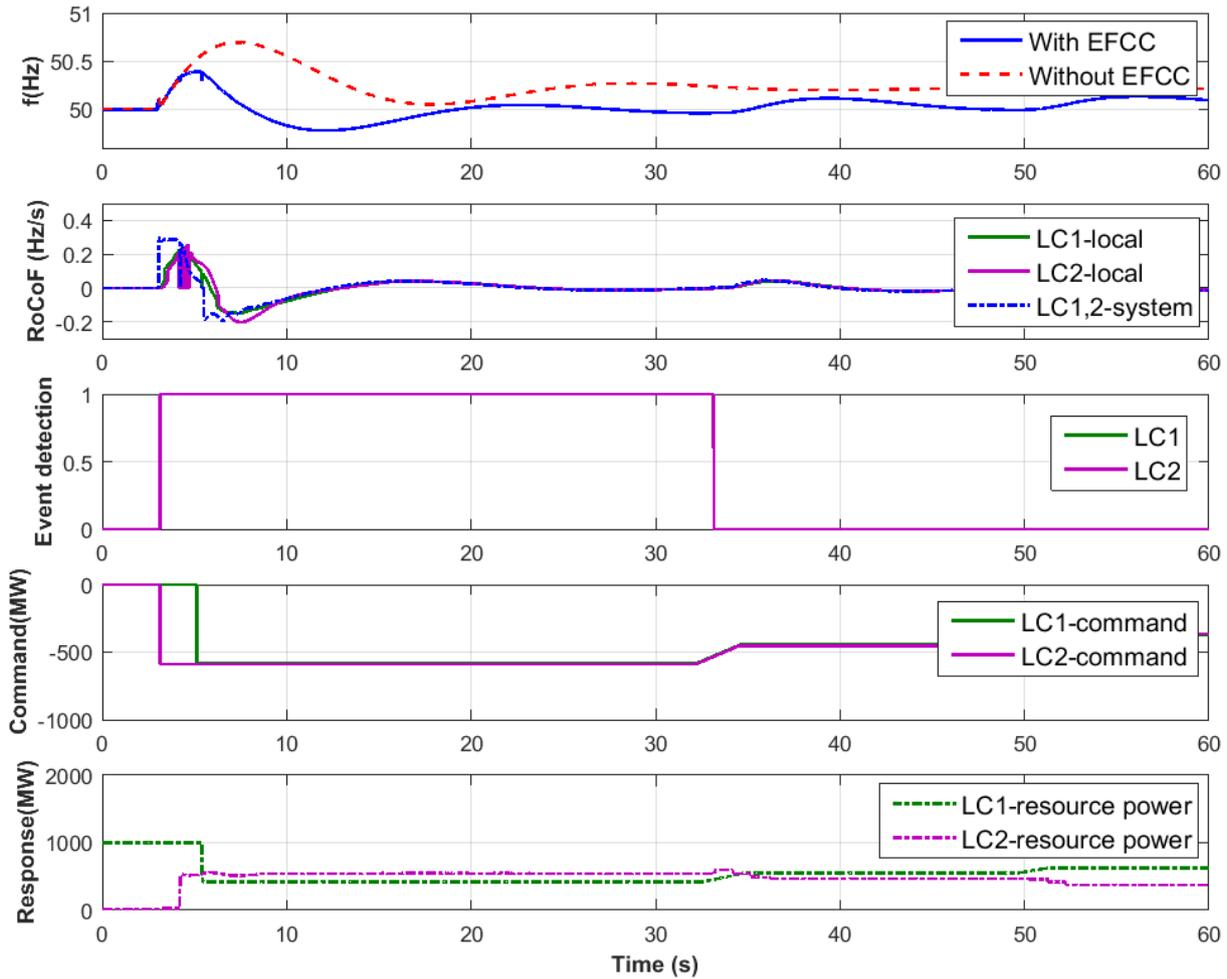
Figure 20. Test 6: over-frequency event test results from LCs
