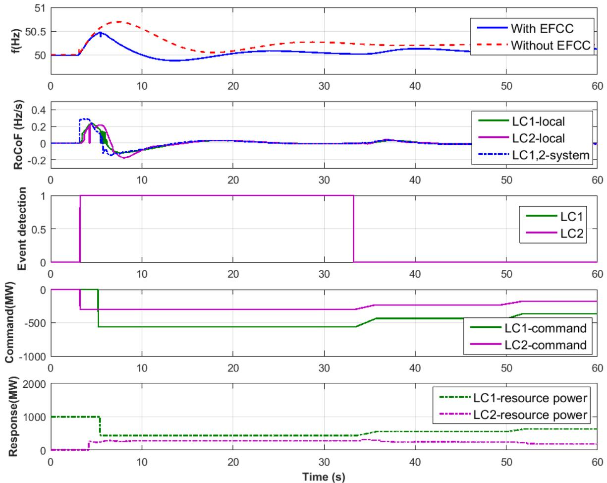
**Figure 32. Test 10: over-frequency event test results from LCs**
