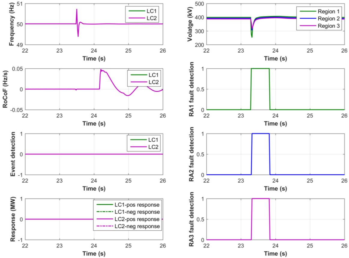
**Figure 56. Test results for a Ph-Ph fault in Region 1**
