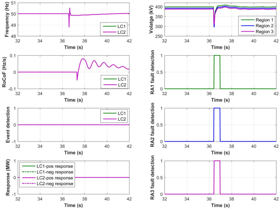
**Figure 59. Test results for a Ph-E fault in Region 2**
