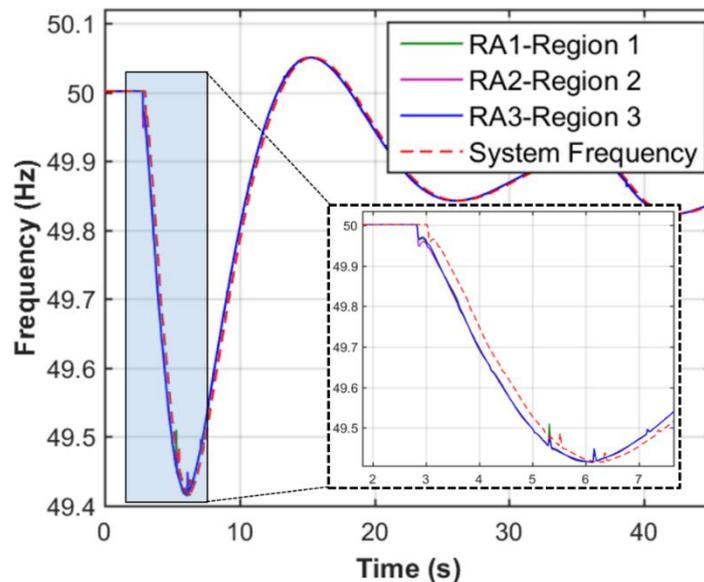
Figure 81. Data recorded in the RAs in the under-frequency test in Test 2
