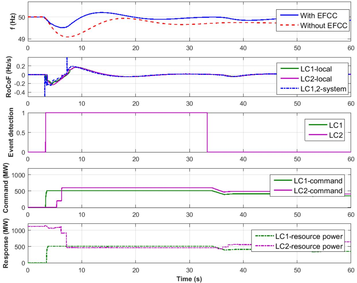
**Figure 40. Test 13 under-frequency event test results from LCs**
