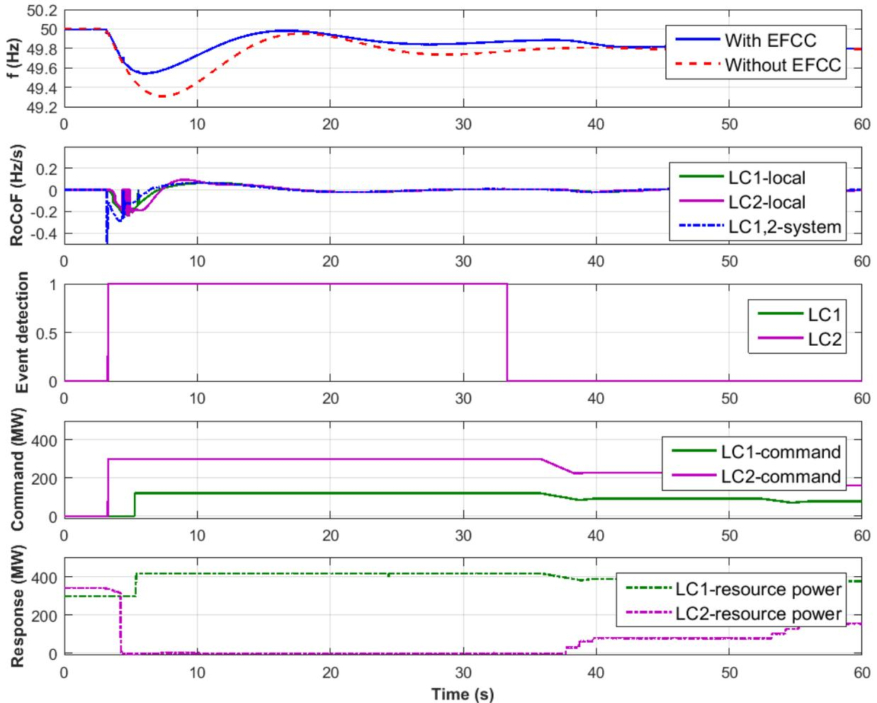
**Figure 4. Test 1: under-frequency event test results from LCs**
