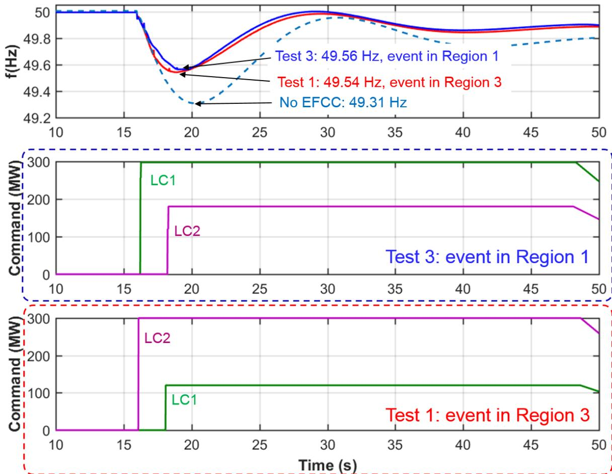
**Figure 49. Comparison of under-frequency test results in Test 1 and Test 3**
