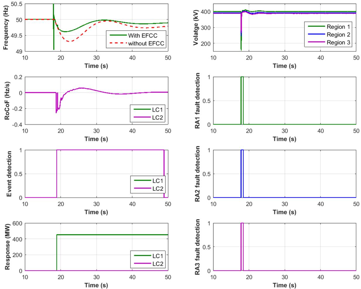
**Figure 67. Test results for a loss of generation event following Ph-Ph fault in Region 1**
