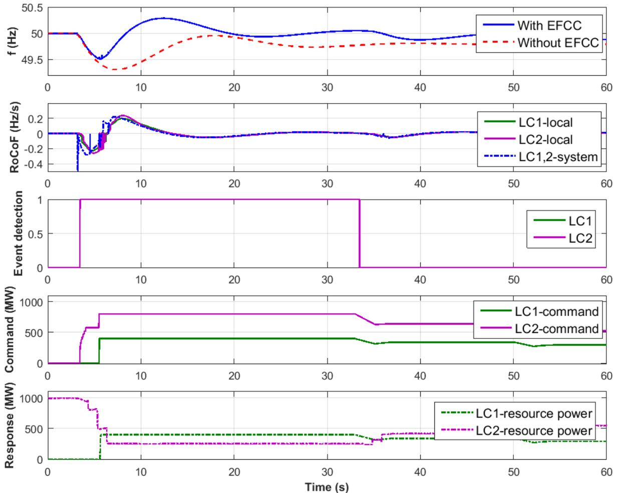
**Figure 19. Test 6: under-frequency event test results from LCs**
