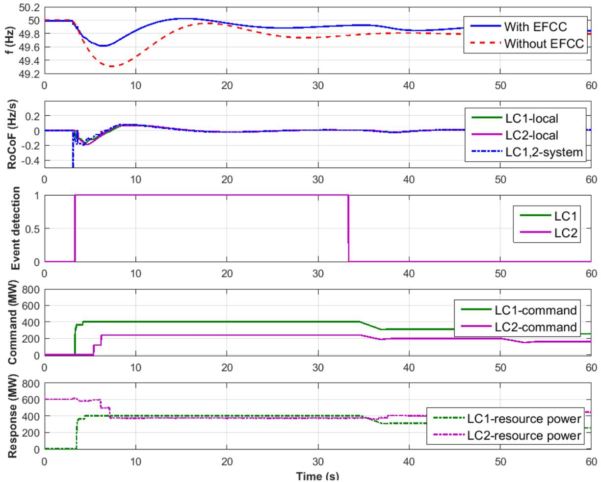
**Figure 16. Test 5: under-frequency event test results from LCs**
