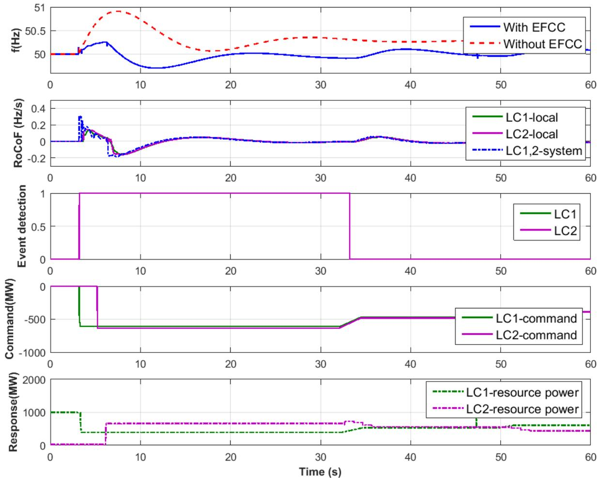
**Figure 41. Test 13: over-frequency event test results from LCs**
