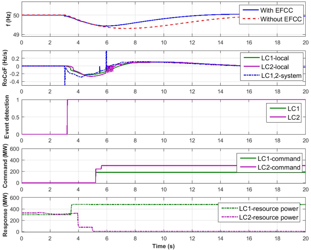
**Figure 46. Test 15: under-frequency event test results from LCs**
