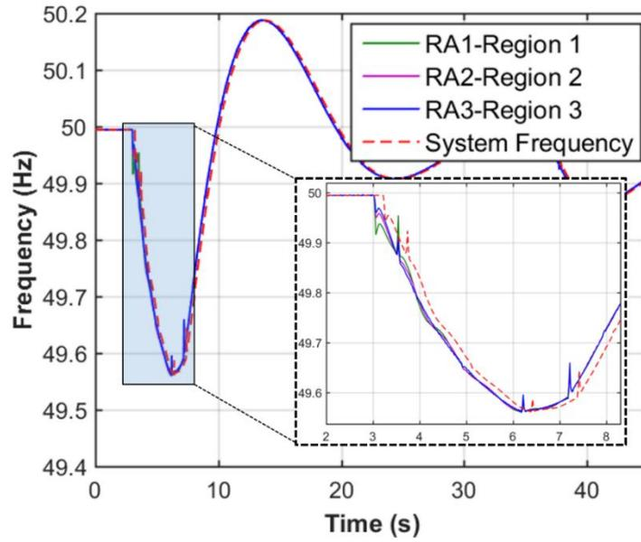
Figure 88. Data recorded in the RAs in the under-frequency test in Test 9
