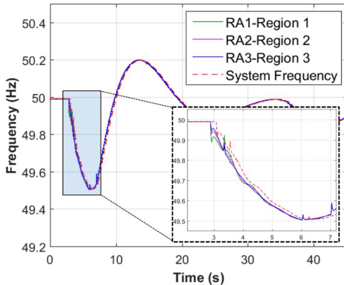
Figure 92. Data recorded in the RAs in the under-frequency test in Test 13
