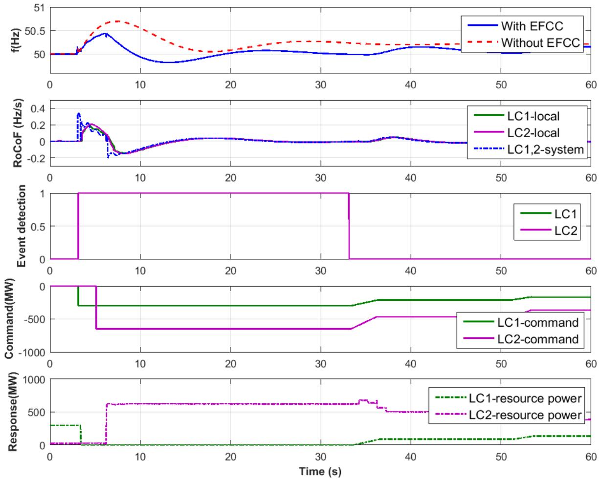
Figure 29. Test 9: over-frequency event test results from LCs
