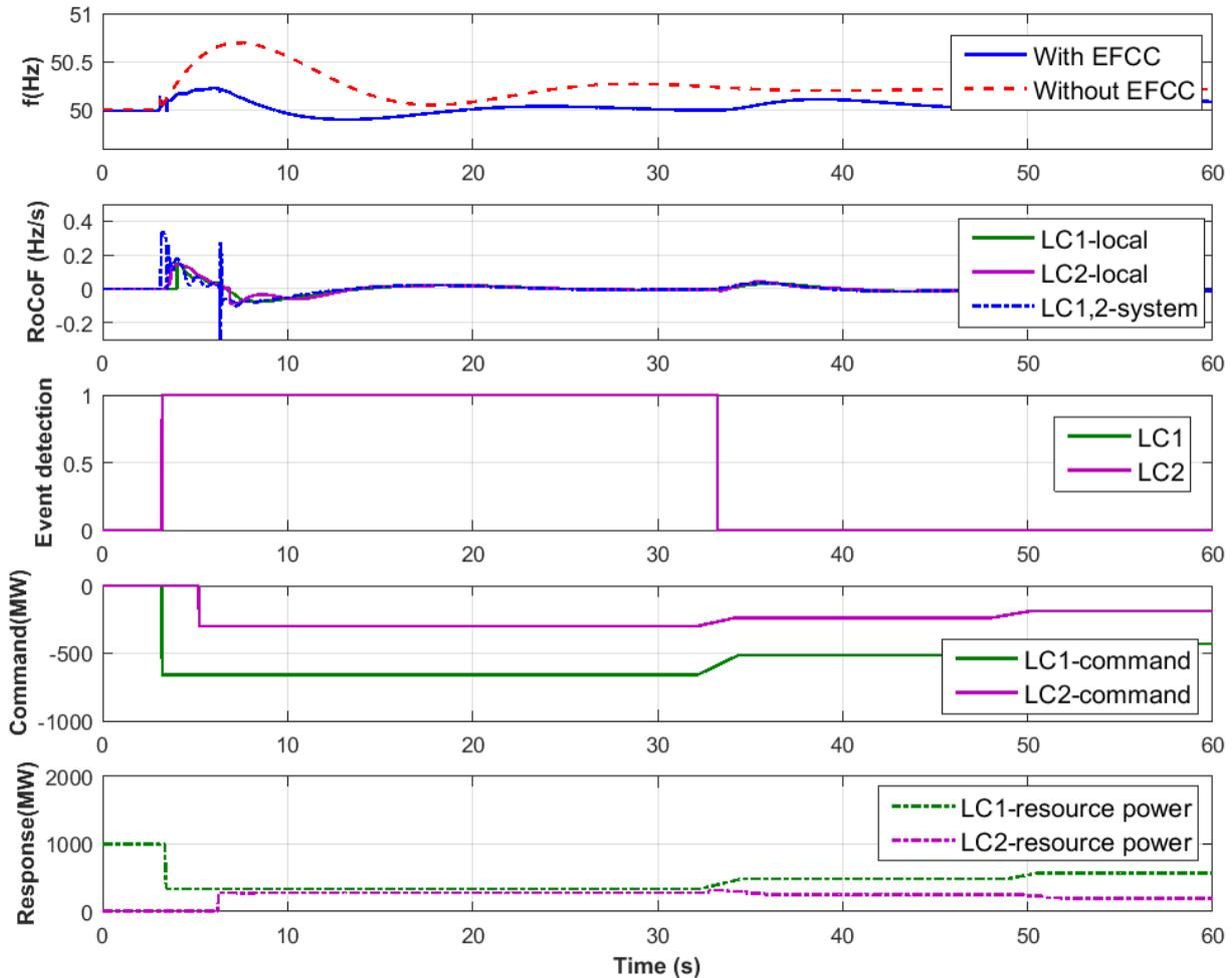
**Figure 35. Test 11: over-frequency event test results from LCs**
