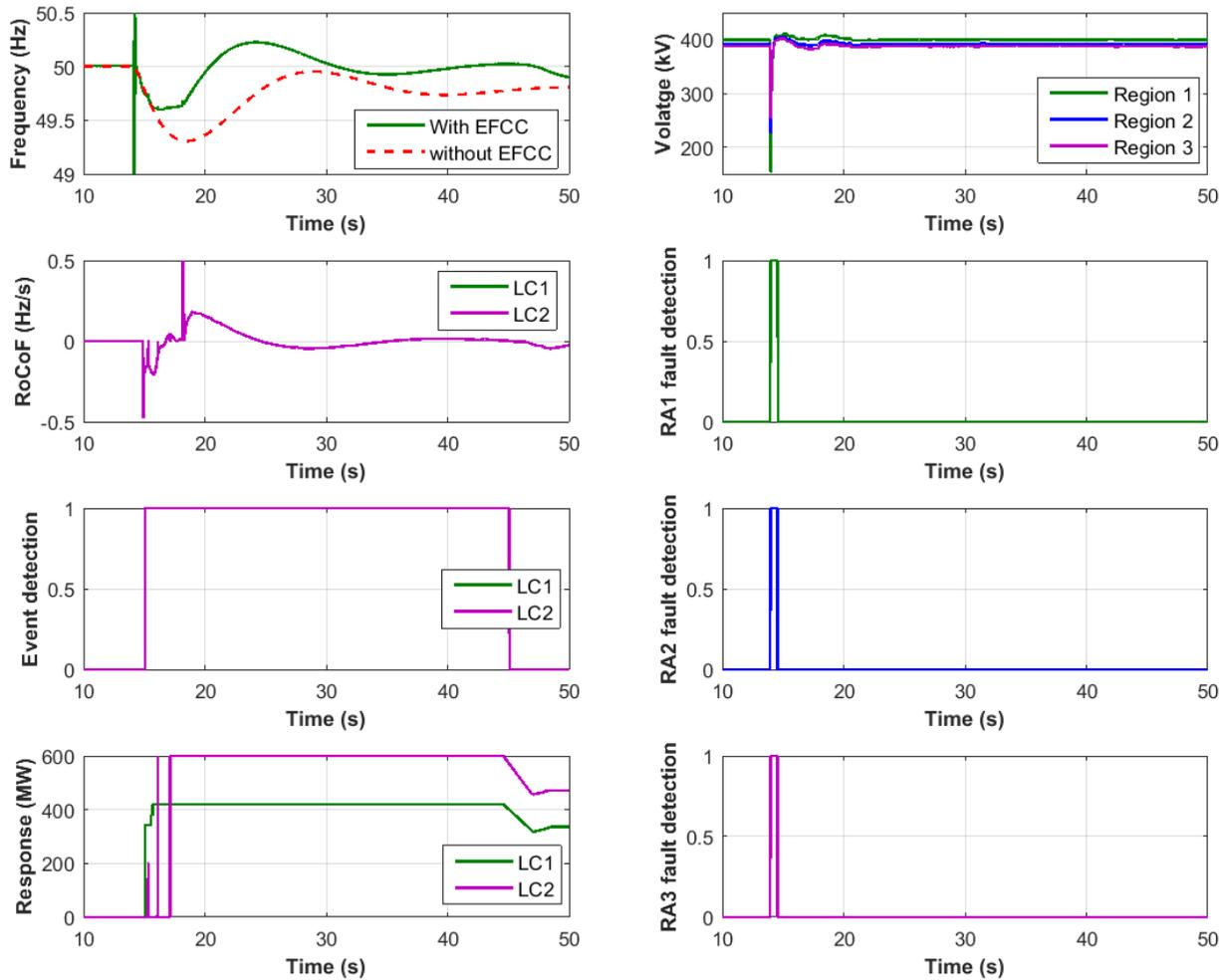
**Figure 68. Test results for a loss of generation event following 3Ph-E fault in Region 1**
