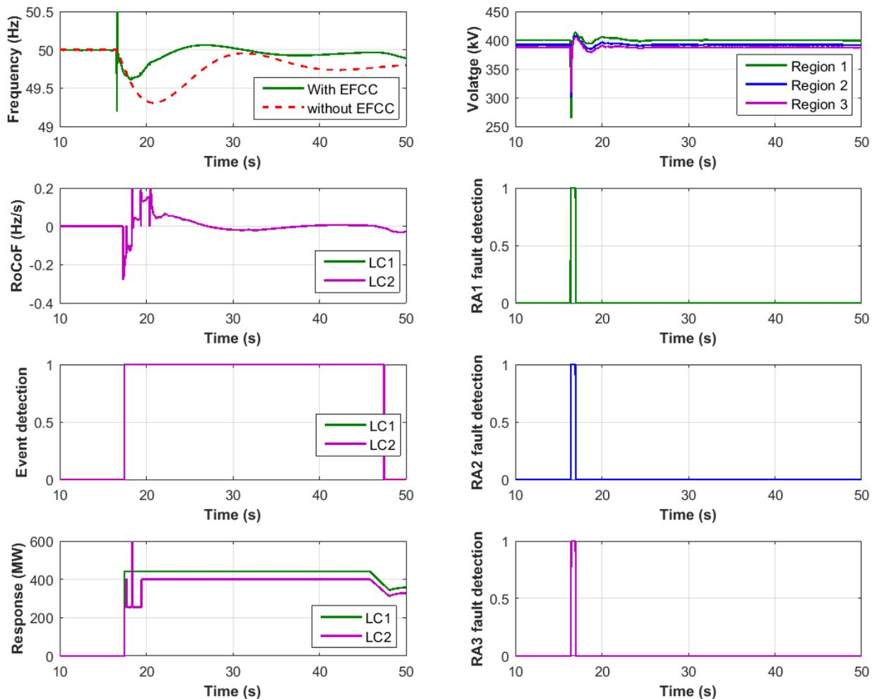
**Figure 66. Test results for a loss of generation event following Ph-E fault in Region 1**
