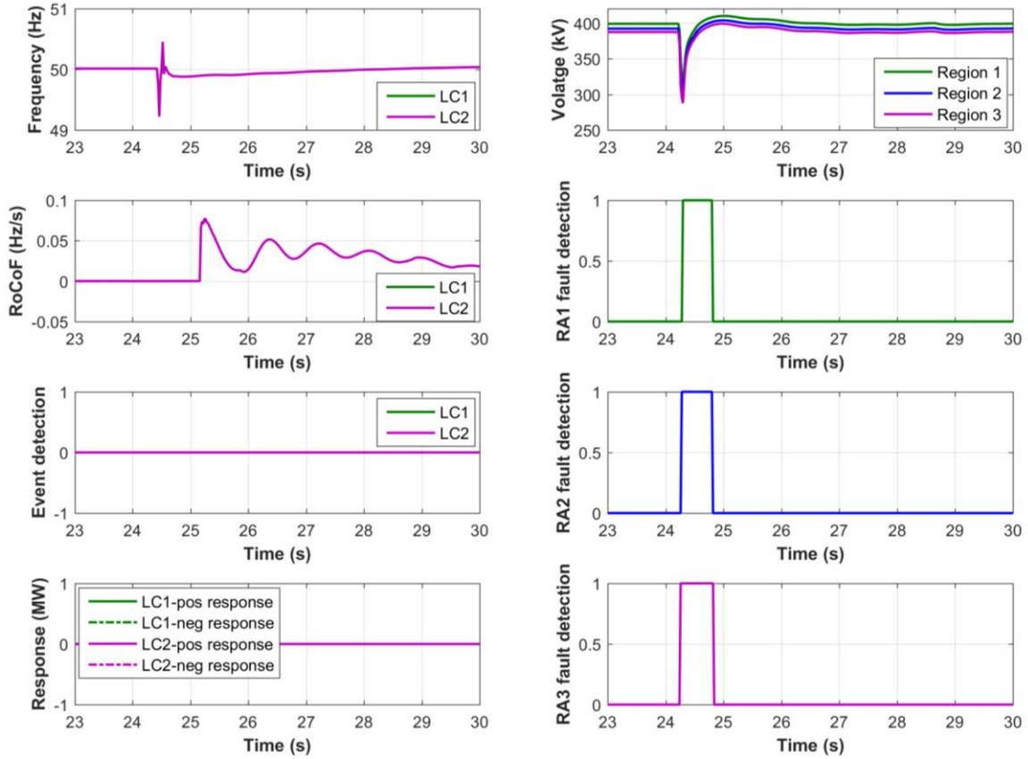
**Figure 63. Test results for a Ph-E fault in Region 3**
