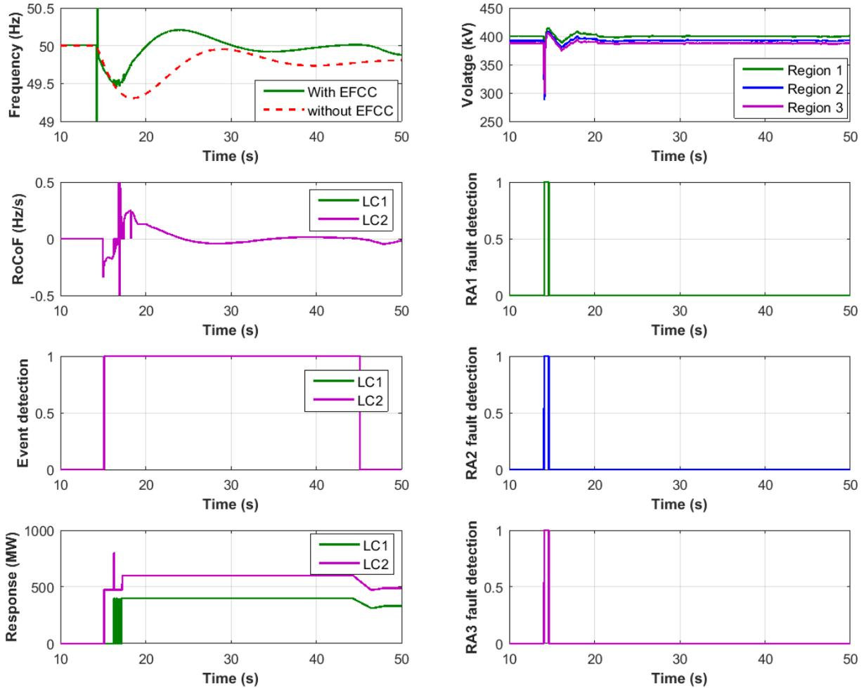
**Figure 69. Test results for a loss of generation event following Ph-E fault in Region 2**
