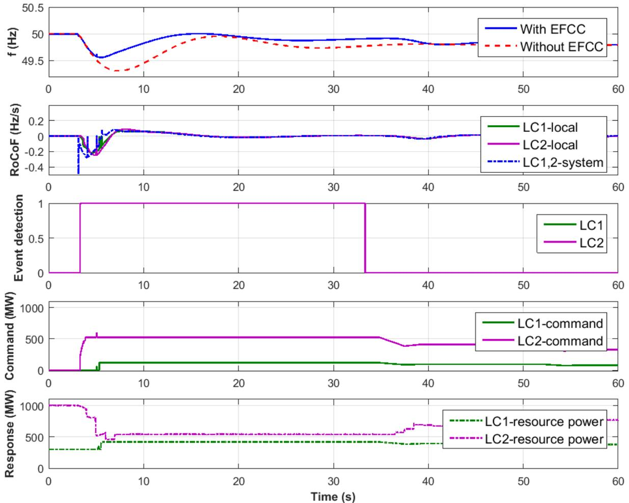
**Figure 25. Test 8: under-frequency event test results from LCs**
