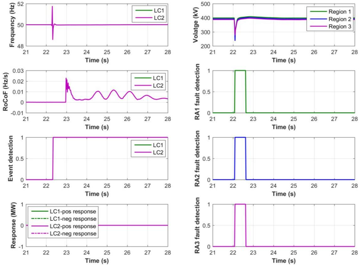
**Figure 60. Test results for a Ph-Ph fault in Region 2**
