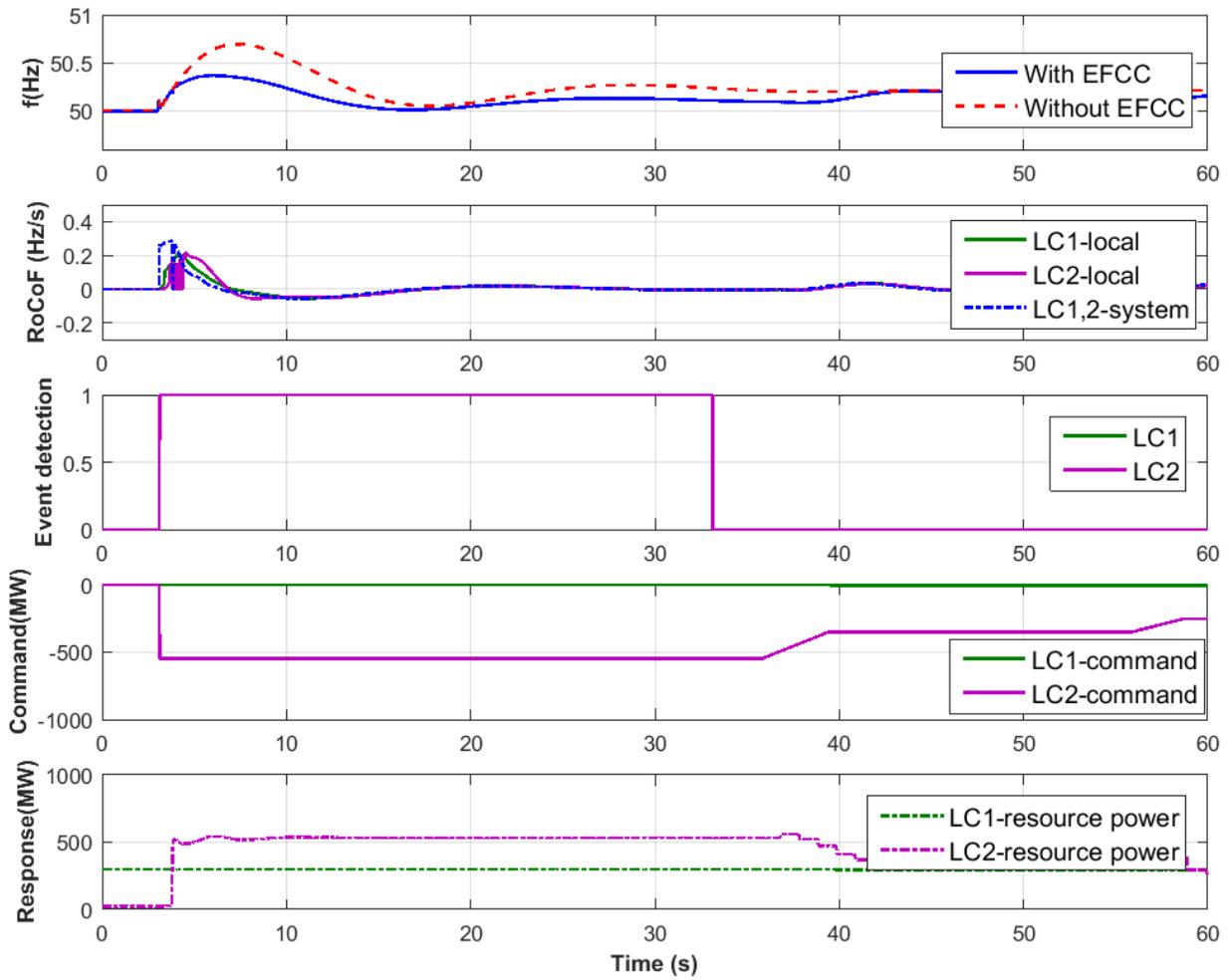
**Figure 26. Test 8: over-frequency event test results from LCs**
