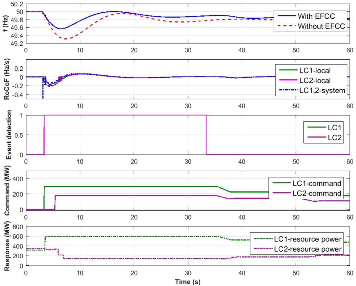
**Figure 10. Test 3: under-frequency event test results from LCs**
