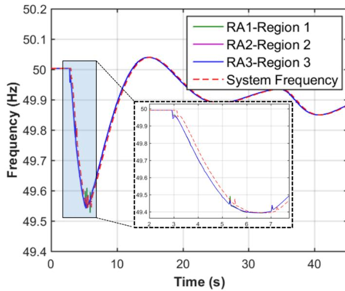
Figure 89. Data recorded in the RAs in the under-frequency test in Test 10
