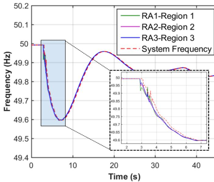
Figure 87. Data recorded in the RAs in the under-frequency test in Test 8
