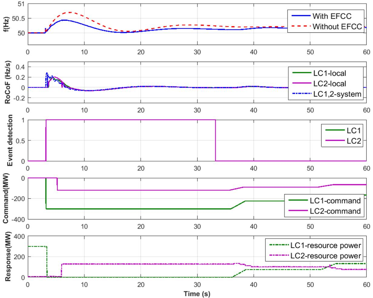
**Figure 11. Test 3: over-frequency event test results from LCs**
