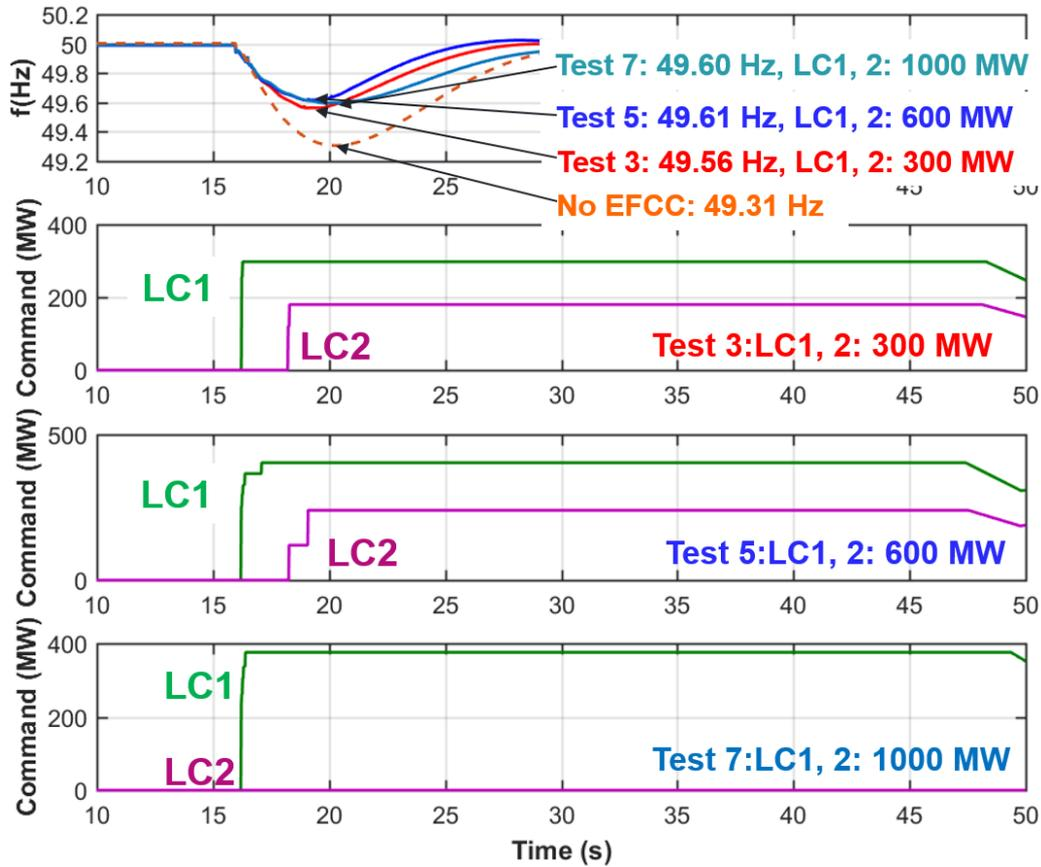
Figure 53. Comparison of under-frequency tests in Test 3, 5 and 7
