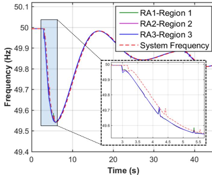
Figure 80. Data recorded in the RAs in the under-frequency test in Test 1
