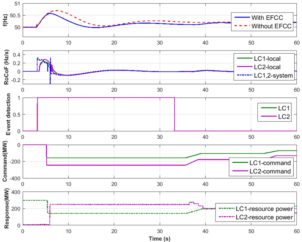
**Figure 8. Test 2: over-frequency event test results from LCs**
