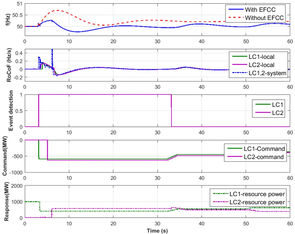
**Figure 23. Test 7: over-frequency event test results from LCs**
