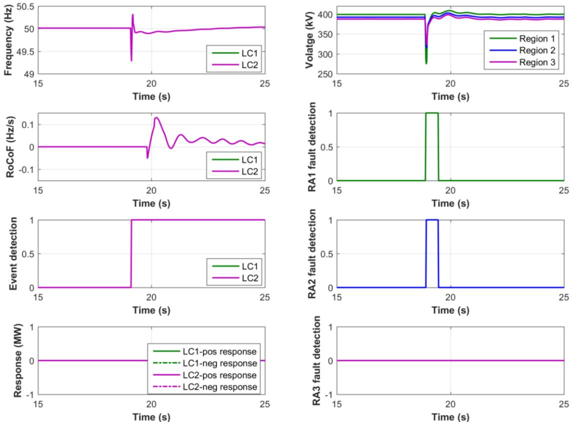
Figure 55. Test results for a Ph-E fault in Region 1
