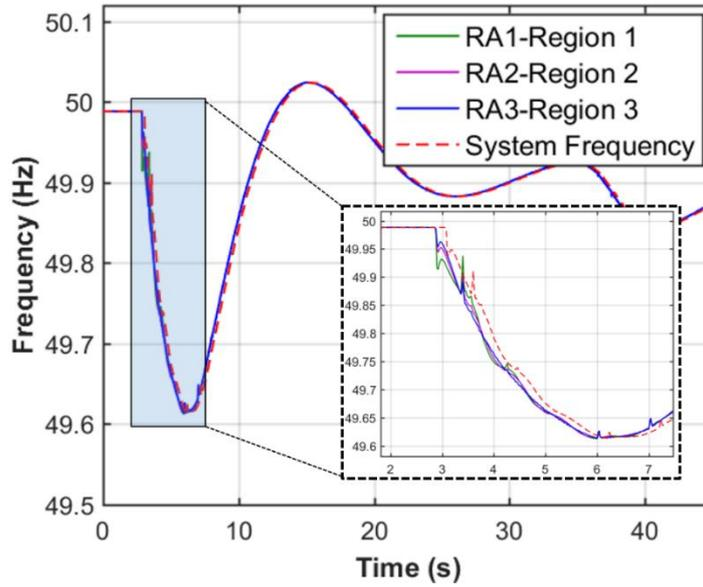
Figure 84. Data recorded in the RAs in the under-frequency test in Test 5
