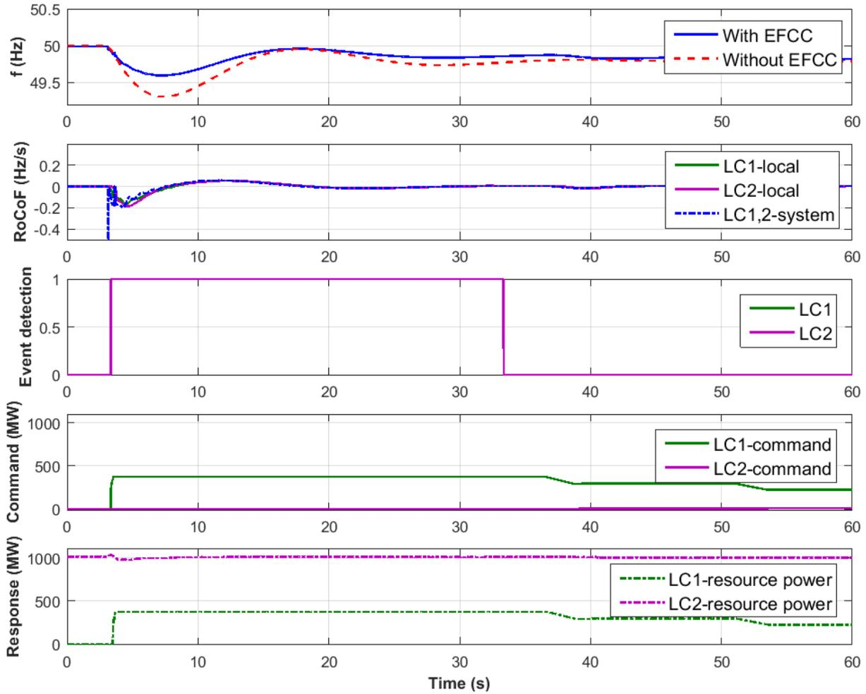
**Figure 22. Test 7: under-frequency event test results from LCs**
