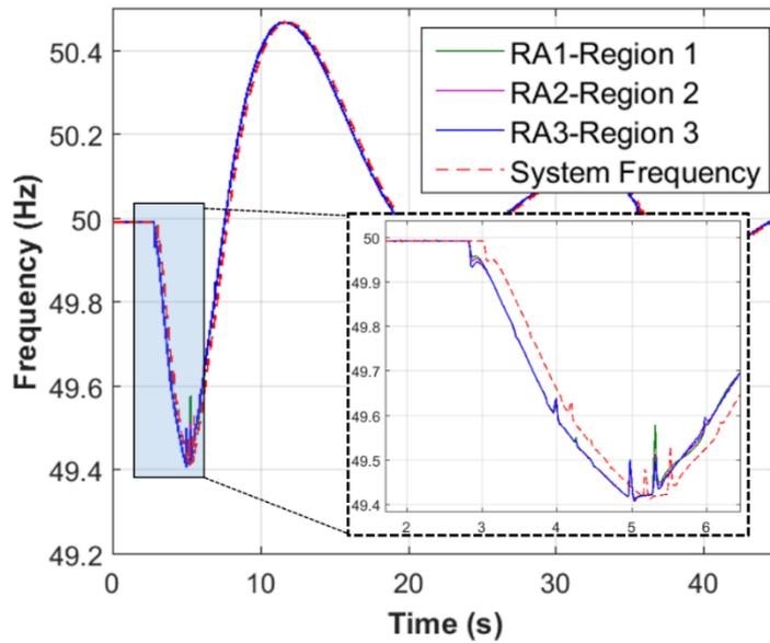
Figure 91. Data recorded in the RAs in the under-frequency test in Test 12
