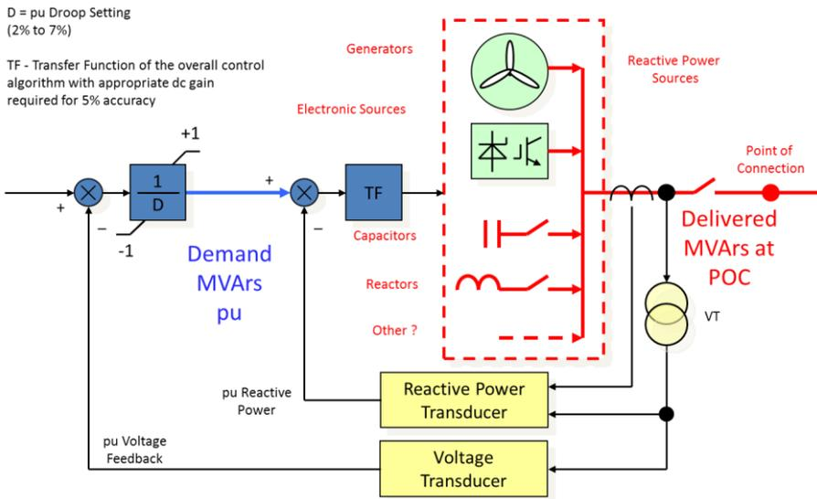
Figure 1: Typical Voltage Control Methodology
