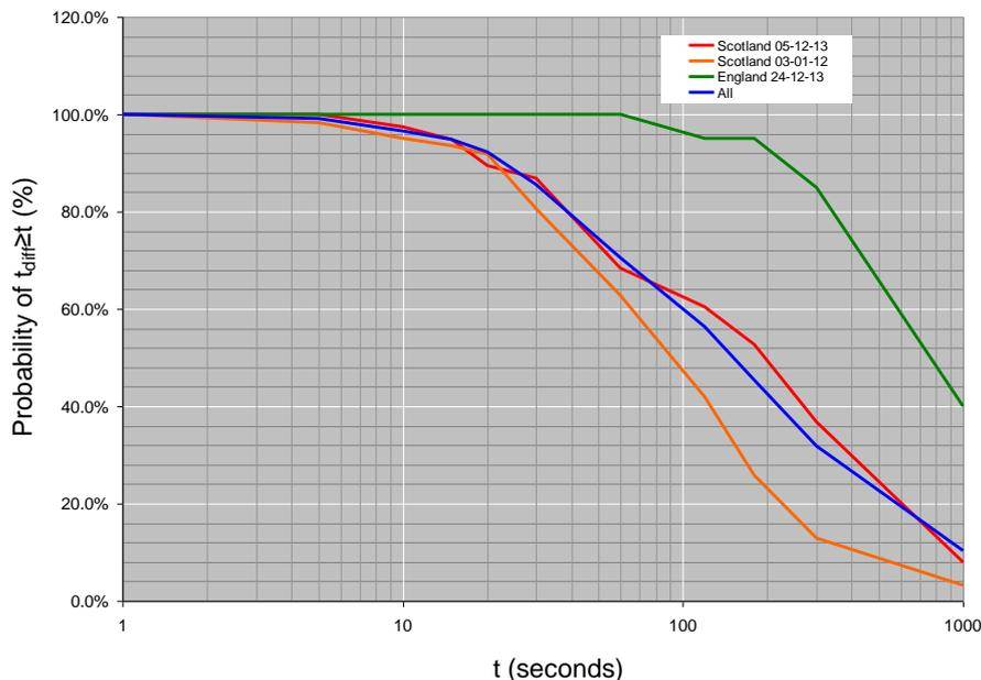
Figure 6: Probability of time difference between two successive events during a storm being greater than a specific value
