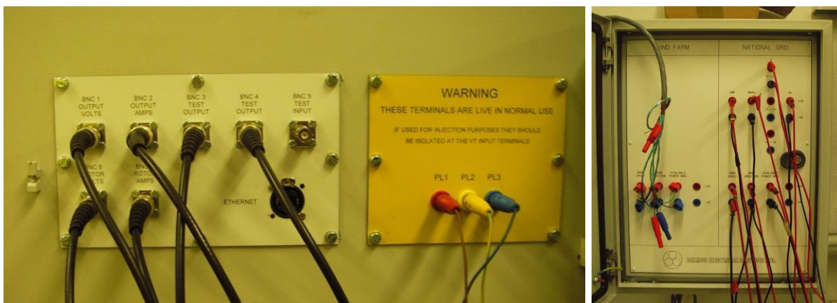
Figure 1: Example of Compliance Test Signal Connections
