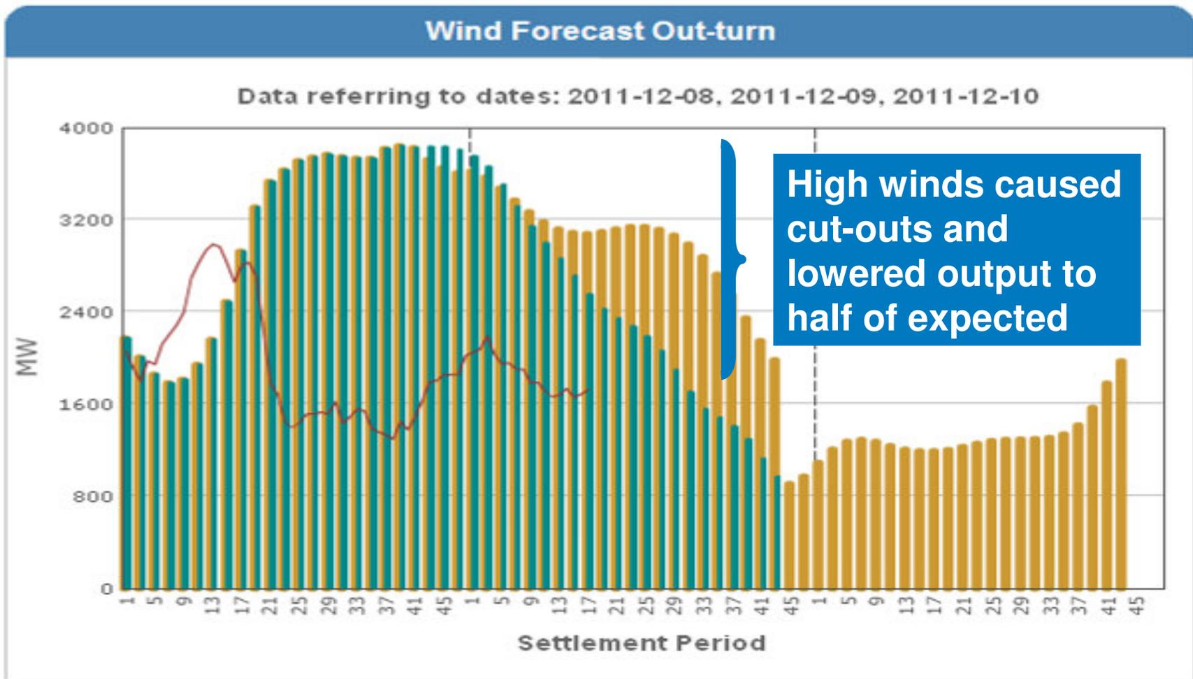
High winds caused cut-outs and lowered output to half of expected
