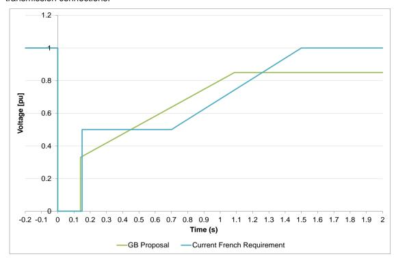
26. Critically, there is the area between 150ms and 450ms where the current French requirement is less onerous than the proposed GB requirement. There is a need to ensure that this area does not cause concern for GB station auxiliaries.
