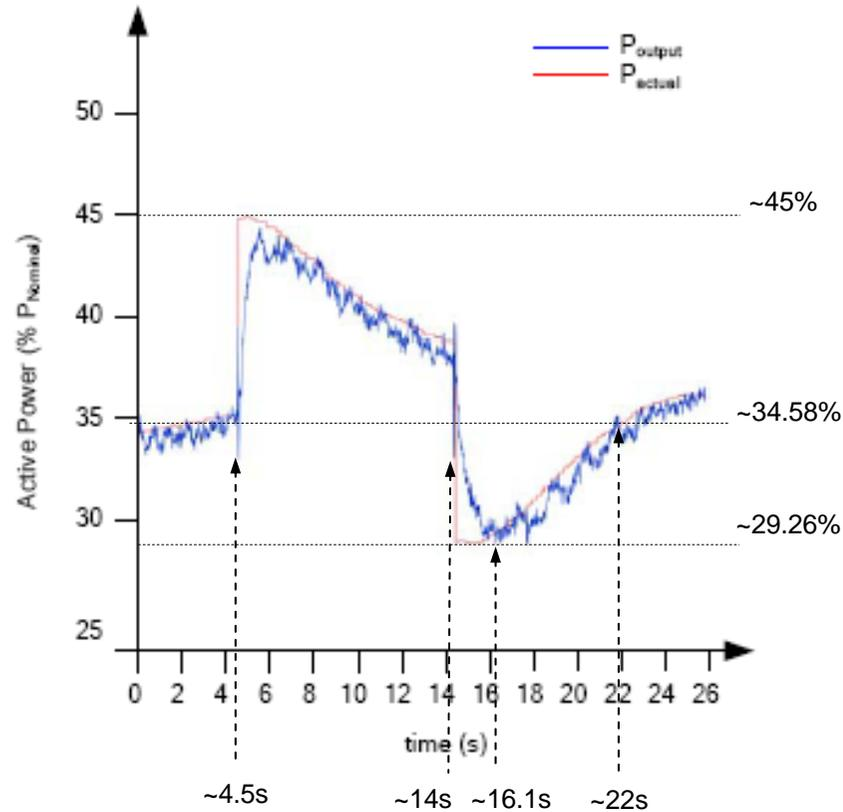
Figure 6 - Power Control including Rotational Speed – Note black dotted lines with extrapolated additional values additional to original figure quoted by Enercon
