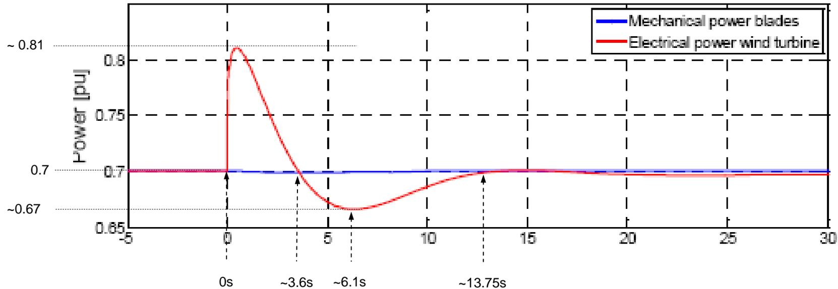
Figure 8 - Wind Power with Inertia emulation – Note black dotted lines with extrapolated additional values additional to original figure quoted by Vestas
